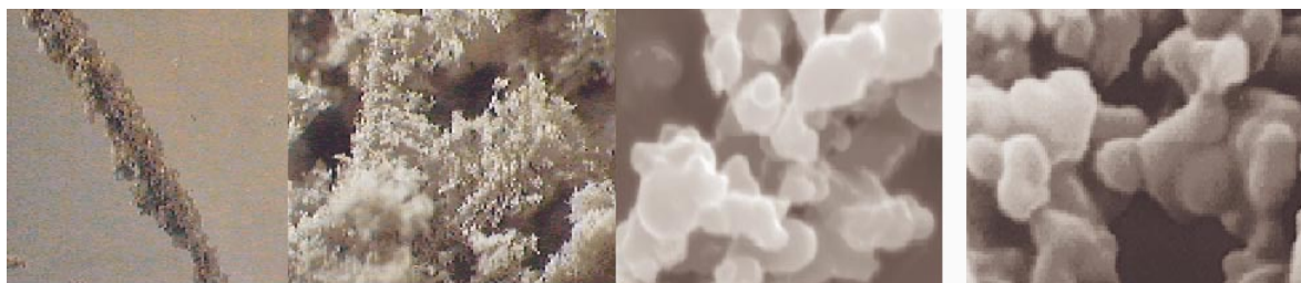
Fig.3 Left part of figure is microscopic photograph of solid product; magnification on left side 150 in middle 500 and on right side SEM photograph with magnification 8000; Right part of figure is SEM photograph of proteinoid protocells published by A.Pappelis & S.Fox [3]
