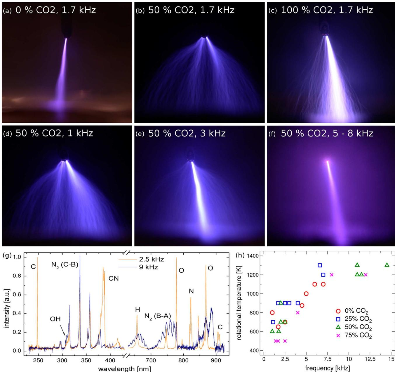
Fig. 1. Photographic images of TS in various gas mixtures and at different frequencies (exposure times: (a)–(c) 1 s and (d)–(f) 4 s). Obtained emission spectra of low- and high-frequency regimes and calculated rotational temperatures as a function of frequency.
