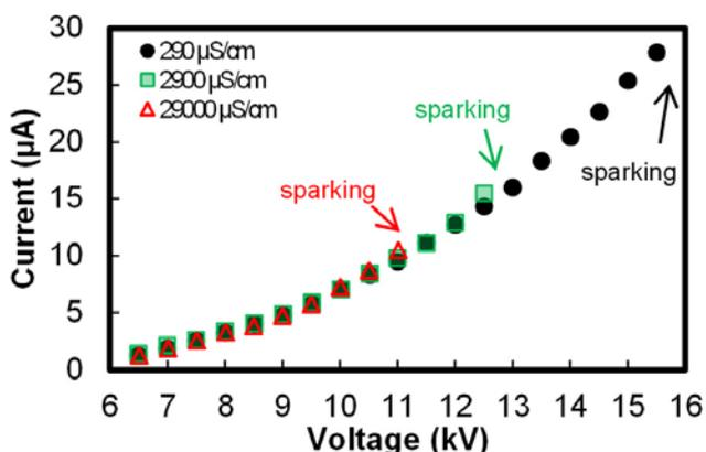
Fig. 3. I-V characteristics of the electro-spray with corona discharge. Different breakdown voltages for corona-to-spark transition are due to different conductivities. [9]
