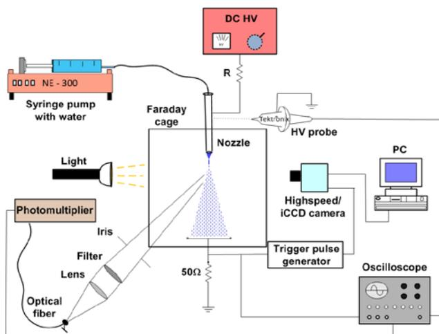
Fig. 1. Experimental set-up for investigations of electrospay of water, with a high-voltage hollow needle (nozzle) electrode enabling water spraying into the discharge.
