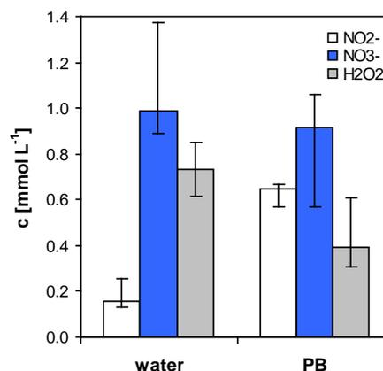
Fig. 4. Nitrite ( $\text{NO}_2^-$ ), nitrate ( $\text{NO}_3^-$ ) and hydrogen peroxide ( $\text{H}_2\text{O}_2$ ) concentrations measured in  $\text{NaH}_2\text{PO}_4$  solution (model tap water, acidification occurs) and PB solution (no acidification occurs) solutions air transient spark plasma treatment via electro-spray. [5]
