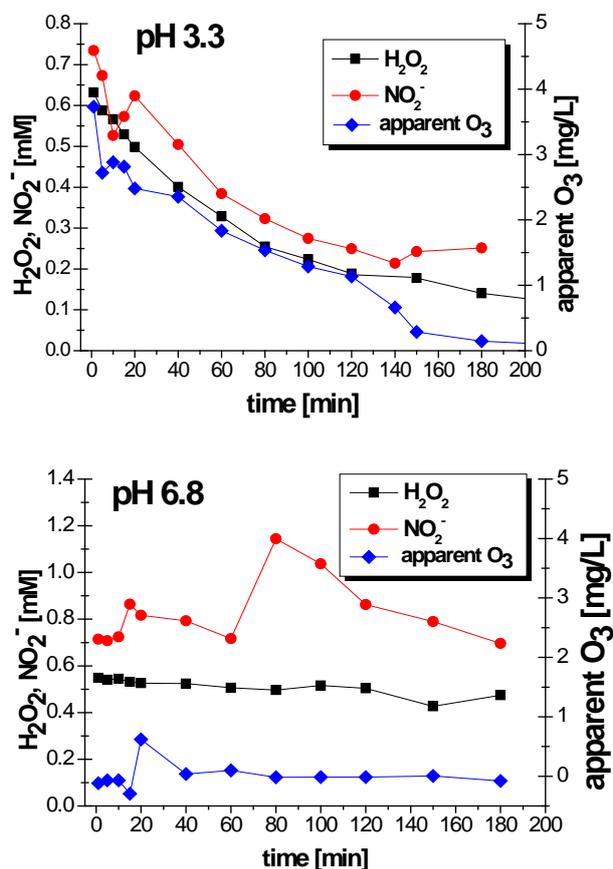
Fig. 5. Time developments of important reactive species in the simulated plasma treated water at pH 3.3 (a) and pH 6.8 (b). Apparent ozone means bleaching of the indigo dye.
