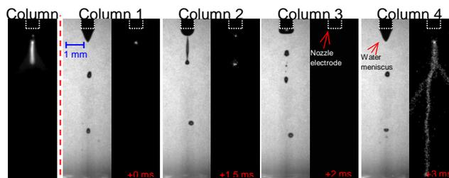
Fig. 2. iCCD time sequence images of electrospay of water (illuminated, columns 1-4 with exposure time 10  $\mu\text{s}$ ) with corona discharge (dark, columns 1-4 with exposure time 100  $\mu\text{s}$ ) in spindle mode for water conductivity 500  $\mu\text{S}/\text{cm}$ , + 6 kV, gap 1 cm, 0.6 mm inner diameter. iCCD dark image in column 0 with exposure time 5 s represents an integrated emission over the long period with many droplet formation cycles. [8]
