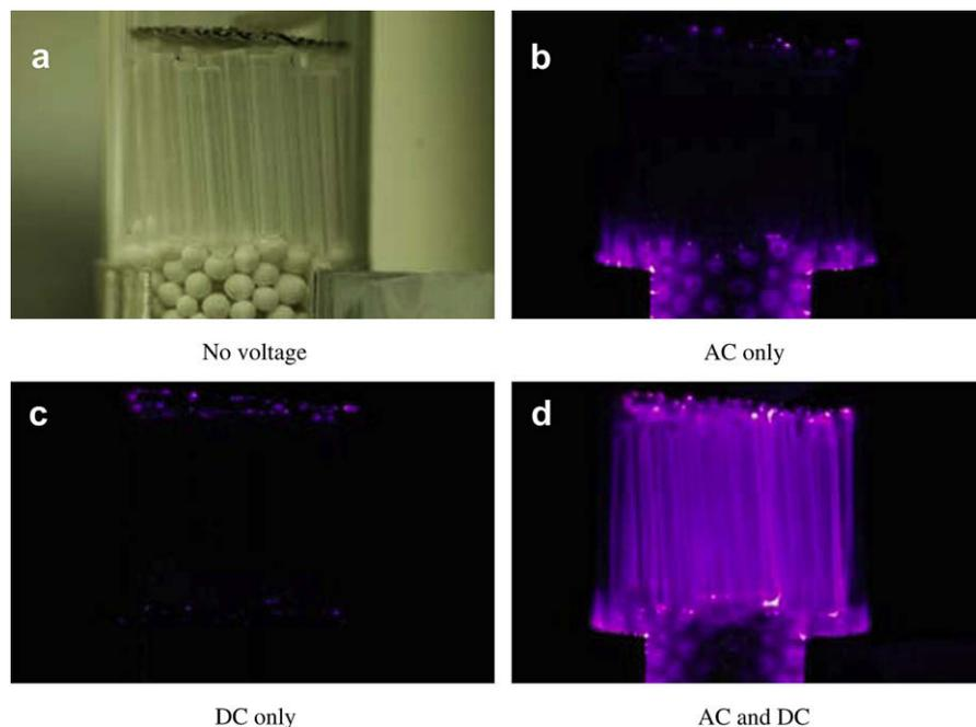
Fig. 3. Photographs of the honeycomb discharge in the bundle of capillary (exposure time of the camera was 6 s). Quartz capillary: 1 mm inner diameter, 20 mm in length, AC 25 kV<sub>p-p</sub>, 1 kHz, DC –11 kV.
