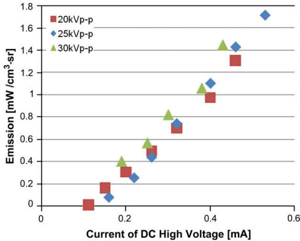
Fig. 11. DC current vs. emission (AC 50 Hz, 2.0 mm inner diameter, 20 mm capillary).
