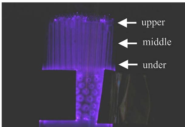
Fig. 12. Photographs of honeycomb discharge (AC 25 kV<sub>p-p</sub> 1 kHz, DC –15 kV 2 mA, N<sub>2</sub> gas 3 L/min, 2.0 mm inner diameter, 20 mm capillary, camera exposure time 4 s).
