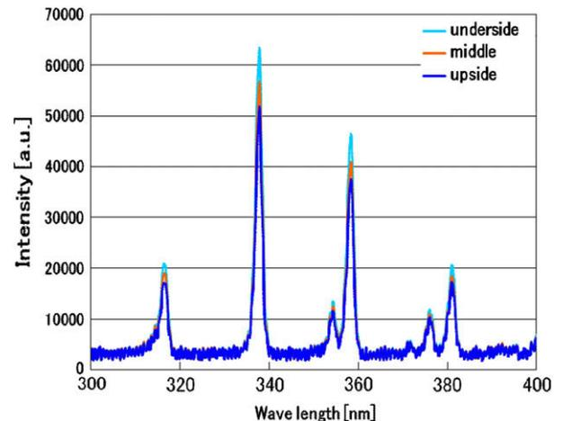
Fig. 13. Wavelength vs. intensity (AC 25 kV<sub>p-p</sub> 1 kHz, DC –15 kV 2 mA, N<sub>2</sub> gas 3 L/min, 2.0 mm inner diameter, 20 mm capillary).
