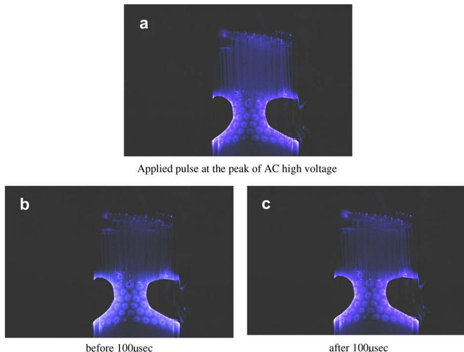
**Fig. 14.** Photographs of the honeycomb discharge using the pulse high voltage. Quartz capillary: 2 mm outer diameter; 20 mm in length; AC 30 kV<sub>p-p</sub>; 1 kHz; pulse –10 kV, 1 kHz; camera exposure time 1.6 s.
