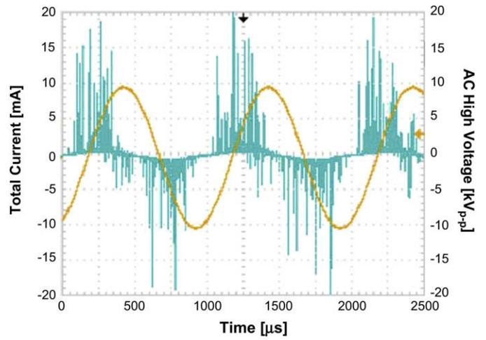
**Fig. 6.** Waveform of AC high voltage and total current for generation of the uniform slide discharge (negative DC high voltage  $-12.5$  kV, AC high voltage  $20$  kV<sub>p-p</sub>,  $2.0$  mm inner diameter,  $20$  mm capillary).
