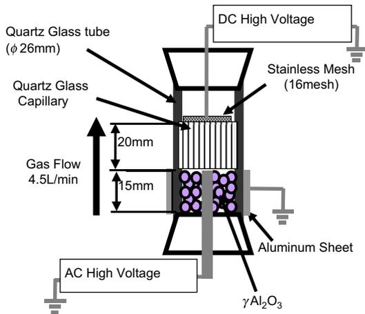
Fig. 1. Schematic diagram of the reactor with bundle of capillary.
