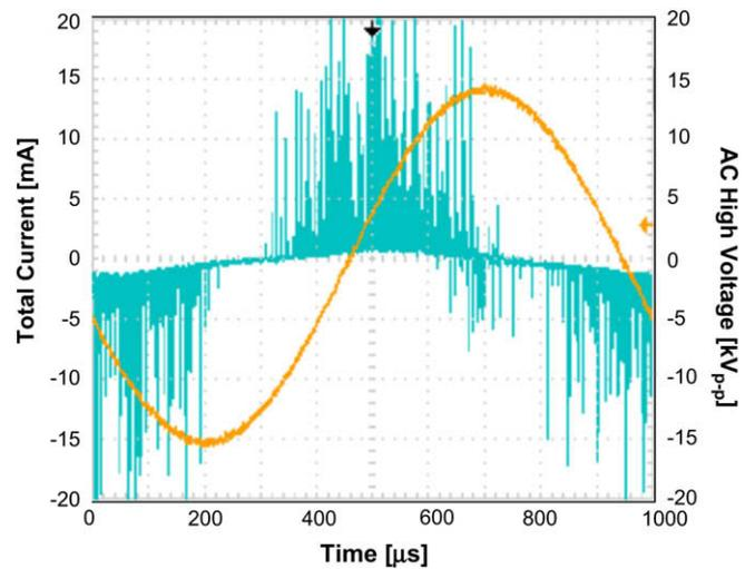
**Fig. 8.** Waveform of AC high voltage and total current for generation of the uniform slide discharge (negative DC high voltage  $-8$  kV, AC high voltage  $30$  kV<sub>p-p</sub>,  $2.0$  mm inner diameter,  $20$  mm capillary).
