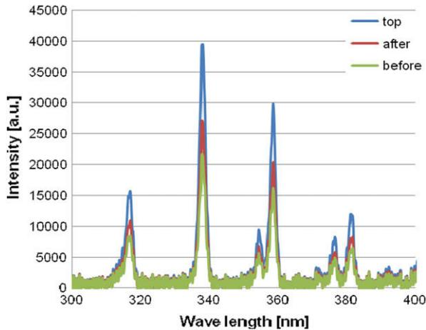
**Fig. 15.** Wavelength vs. emission intensity (AC 30 kV<sub>p-p</sub> 1 kHz, pulse –10 kV, 1 kHz, air 3 L/min, 2.0 mm inner diameter, 20 mm capillary).
