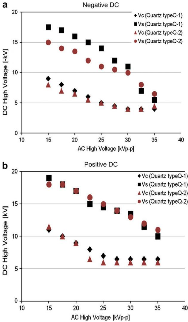
**Fig. 4.** Relationship between DC and AC high voltage for generation of the uniform discharge plasma. Capillary length, 20 mm; Q-1, 1.0 mm; Q-2, 2.0 mm inner diameter; Vc, the starting voltage; Vs, the maximum voltage (the flashover voltage).
