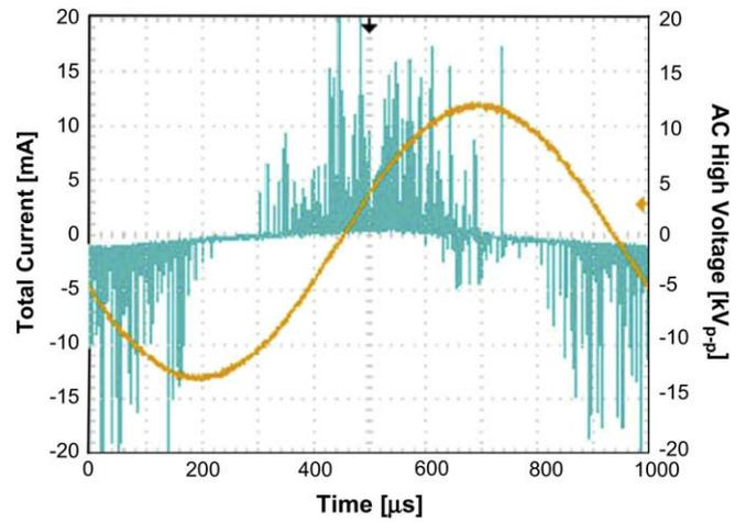
**Fig. 7.** Waveform of AC high voltage and total current for generation of the uniform slide discharge (negative DC high voltage  $-10$  kV, AC high voltage  $25$  kV<sub>p-p</sub>,  $2.0$  mm inner diameter,  $20$  mm capillary).
