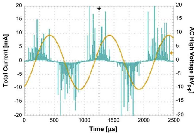
**Fig. 5.** Waveform of AC high voltage and total current for generation only packed bed discharge (negative DC high voltage  $0$  kV,  $2.0$  mm inner diameter, AC high voltage  $20$  kV<sub>p-p</sub>,  $20$  mm capillary).
