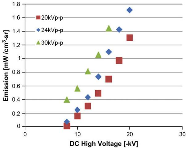
Fig. 9. DC high voltages vs. emission (AC 50 Hz, 2.0 mm inner diameter, 20 mm capillary).
