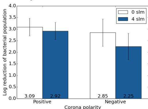
Fig. 4. Logarithmic reduction of bacterial population by the corona discharges with or without blowing of air through the discharge, exposure time 5 min (5-8 repeats, mean±SD).
