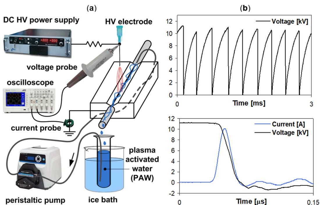
**Figure 1.** (a) The scheme of experimental setup and (b) characteristic voltage and current waveforms of self-pulsing transient spark discharge in two different timescales.
