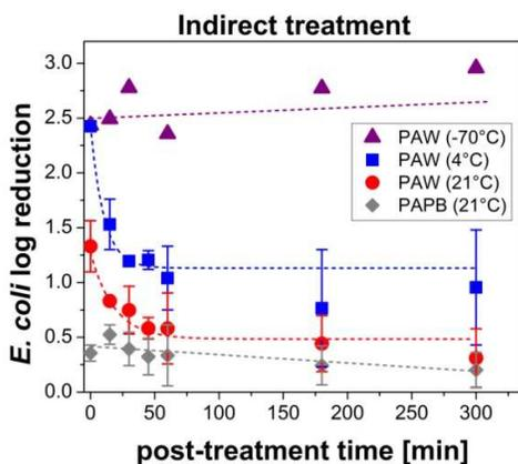
**Fig. 3.** Post-plasma treatment evolution of bactericidal properties of plasma activated solutions stored at different temperatures (indirect treatment - each point represents 10 min incubation; mean, 1<sup>st</sup> and 3<sup>rd</sup> quartile).
