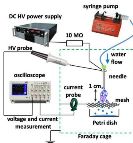
Fig. 1. Experimental set-up of air transient spark with water electrospray.
