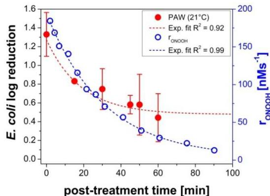
**Fig. 4.** Correlation of the exponential decay of bactericidal effect of PAW and the rate constant of ONOOH formation ( $r_{\text{ONOOH}}$ ) in PAW in post-plasma treatment (at room temperature).
