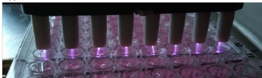
**Figure 1** Treatment of cancer cells in 96-well plate in multiple streamer corona setup.
