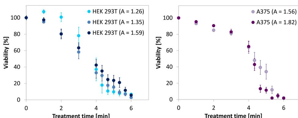
Viability of normal HEK 293T and cancer A375 cells in dependence on SC discharge treatment time after 24 hours incubation. The "A" value refers to the absorbance of control sample which is proportional to initial metabolic activity of cells.
