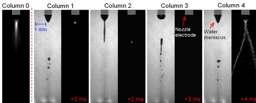
**Figure 9.** iCCD time sequence images of electro spraying of water (illuminated, columns 1–4 with exposure time  $10 \mu\text{s}$ ) with corona discharge (dark, columns 1–4 with exposure time  $100 \mu\text{s}$ ) in spindle mode for water conductivity  $4 \mu\text{S cm}^{-1}$ , +6 kV, gap 1 cm, nozzle 0.8 mm o.d. and 0.6 mm i.d. iCCD dark images in column 0 with exposure time 5 s represent an integrated emission over the long period with many droplet formation cycles.
