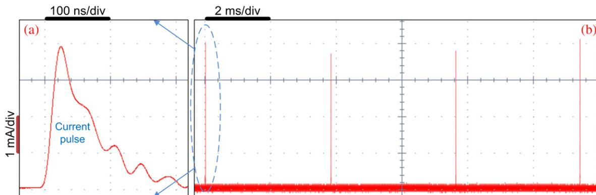
**Figure 5.** Oscilloscopic waveform of the discharge current pulses during the electro spraying of water in spindle mode. Image (a) corresponds to one current pulse in high time resolution 100 ns/div, image (b) corresponds to the many current pulses in low time resolution 2 ms/div (6 kV, conductivity  $2 \mu\text{S cm}^{-1}$ , gap 1 cm, nozzle 0.7 mm o.d., 0.5 mm i.d., water flow rate  $0.4 \text{ ml min}^{-1}$ ).
