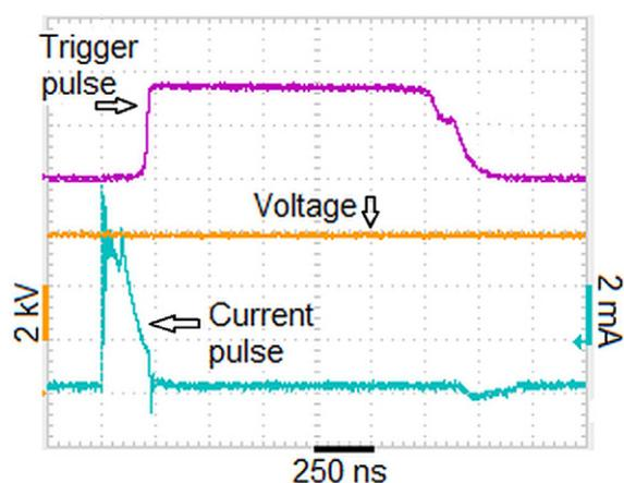
**Figure 2.** Oscilloscopic records of the discharge voltage and current pulse, and the pulse triggering the iCCD camera during the electrospaying of water.
