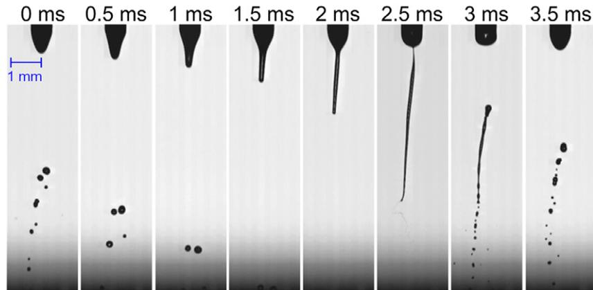
**Figure 3.** HS camera sequence of electro spraying of deionized water in spindle mode (6 kV, conductivity  $2 \mu\text{S cm}^{-1}$ , gap 1 cm, nozzle 0.7 mm o.d., 0.5 mm i.d., water flow rate  $0.4 \text{ ml min}^{-1}$ , time step  $500 \mu\text{s}$ ).
