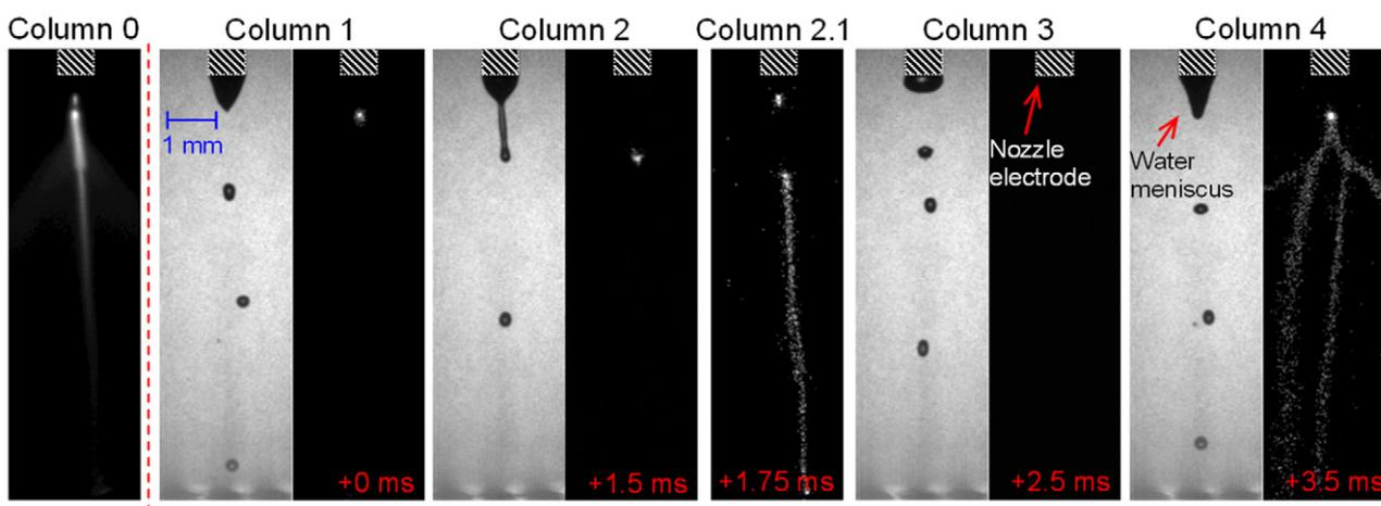
**Figure 11.** iCCD time sequence images of electro spraying of water (illuminated, columns 1–4 with exposure time  $10 \mu\text{s}$ ) with corona discharge (dark, columns 1–4 with exposure time  $100 \mu\text{s}$ ) in spindle mode for water conductivity  $4500 \mu\text{S cm}^{-1}$ , +6 kV, gap 1 cm, nozzle 0.8 mm o.d. and 0.6 mm i.d. iCCD dark images in column 0 with exposure time 5 s represent an integrated emission over the long period with many droplet formation cycles.
