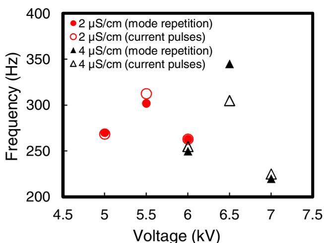
**Figure 6.** Comparison of mode repetition (filled markers) frequencies measured by HS or iCCD camera and the frequencies of current pulses (open markers) for various voltages and low water conductivities.
