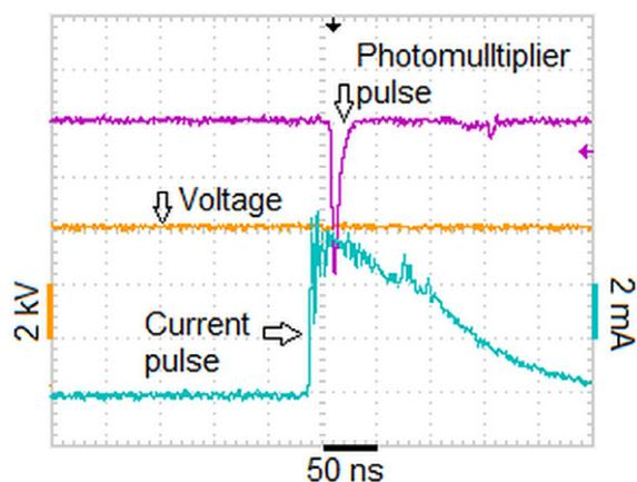
**Figure 8.** Oscilloscopic records of the discharge voltage, current pulse, and the PMT pulse (6 kV, conductivity  $500 \mu\text{S cm}^{-1}$  gap 1 cm, nozzle 0.8 mm o.d., 0.6 mm i.d.).
