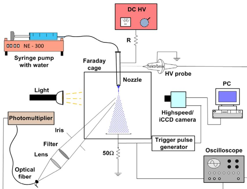
**Figure 1.** Experimental set-up for investigations of the electrospay of water, with a HV hollow needle (nozzle) electrode enabling water flow into the inter-electrode space.
