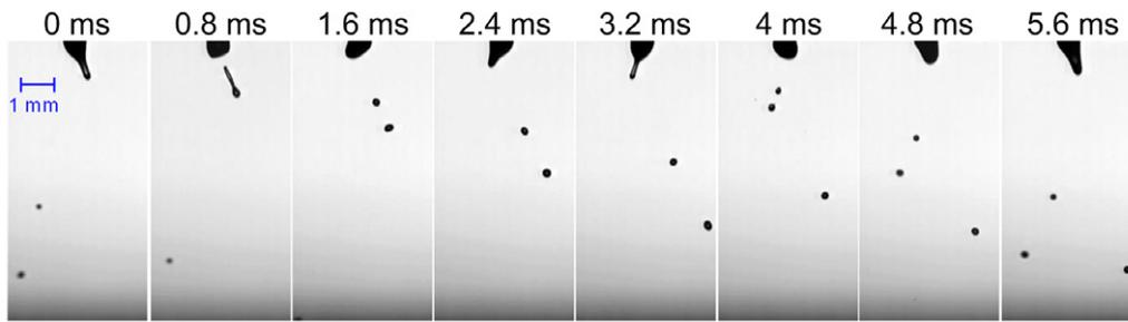
**Figure 4.** HS camera sequence of electrospaying of water in oscillating-spindle mode (6 kV, conductivity  $400 \mu\text{S cm}^{-1}$ , gap 1 cm, nozzle 0.7 mm o.d., 0.5 mm i.d., water flow rate  $0.4 \text{ ml min}^{-1}$ , time step  $800 \mu\text{s}$ ).
