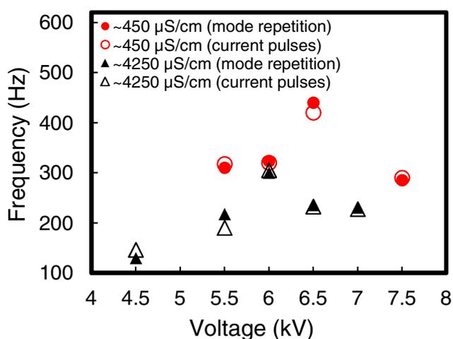
**Figure 7.** Comparison of mode repetition (filled markers) frequencies measured by HS or iCCD camera and the frequencies of current pulses (open markers) for various voltages and water solutions of high conductivities.
