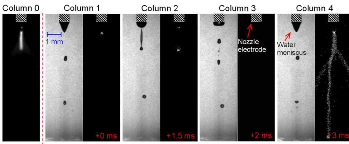
**Figure 10.** iCCD time sequence images of electro spraying of water (illuminated, columns 1–4 with exposure time  $10 \mu\text{s}$ ) with corona discharge (dark, columns 1–4 with exposure time  $100 \mu\text{s}$ ) in spindle mode for water conductivity  $500 \mu\text{S cm}^{-1}$ , +6 kV, gap 1 cm, nozzle 0.8 mm o.d. and 0.6 mm i.d. iCCD dark images in column 0 with exposure time 5 s represent an integrated emission over the long period with many droplet formation cycles.
