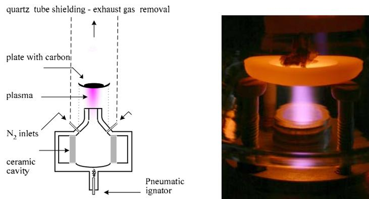
**Figure 3.** Treatment of carbon samples.
