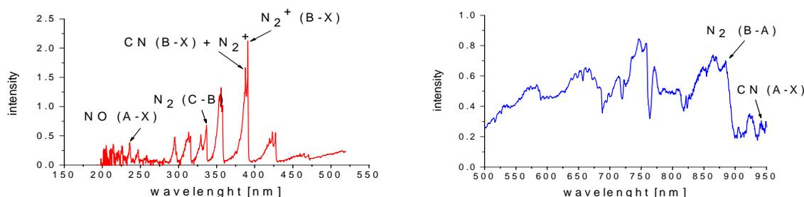
**Figure 4.** Measured spectra in UV and VIS region.
