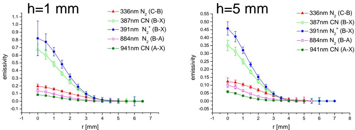
**Figure 5.** Abel-inverted horizontal profiles in  $h=1$  mm and  $h=5$  mm.
