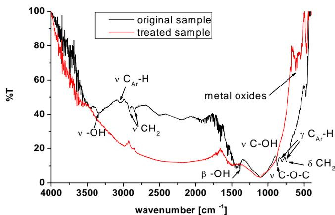
**Figure 7.** FTIR spectra of carbon samples.
