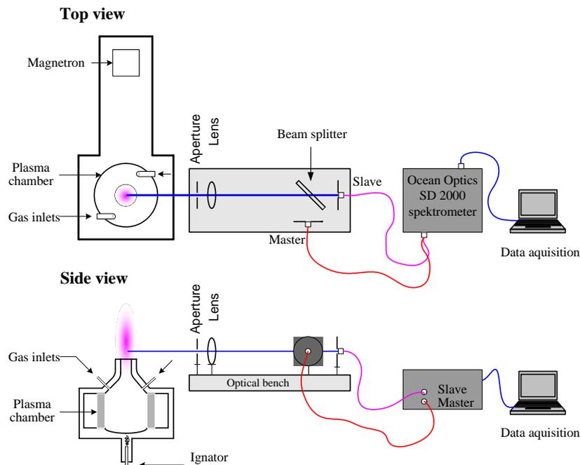
**Figure 2.** Experimental setup.
