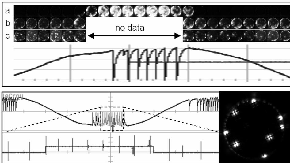
**Fig.2.** Light emission of the discharges synchronized with the AC high voltage signal. Parameters: pore size  $80\mu\text{m}$ , nitrogen, applied voltage  $15.7\text{ kV}$ , intensifier gate  $500\ \mu\text{s}$ . Series: a) intensifier sensitivity 500, integration 100x, b) intensifier sensitivity 600, integration 100x, c) intensifier sensitivity 760.
