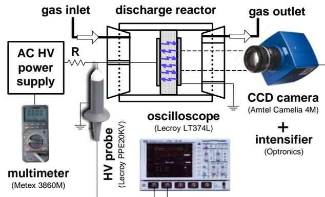
Fig. 1. Simplified sketch of the experimental setup.
