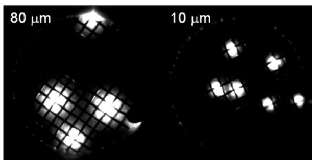
**Fig.4.** Comparison of the microdischarges in various ceramics. Parameters: nitrogen, applied voltage  $\sim 16\text{ kV}$ , intensifier gate 1ms, intensifier sensitivity 420.
