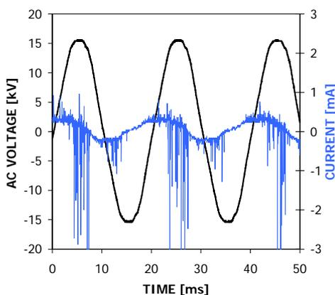
Fig. 2. Waveforms of the applied voltage and discharge current of sliding discharge [ $U_{AC} = 15$  kV,  $U_{DC} = -16$  kV]
