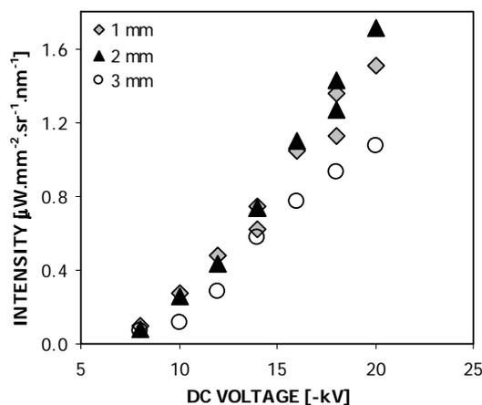
Fig. 7. Emission intensity as functions of negative DC applied voltage for various diameters of capillaries [length 20 mm, AC 10 kV]
