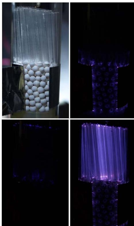
Fig. 3. Images of the discharge in capillaries [diameter 2 mm, length 3 mm] at different AC and DC applied voltages in ambient air: (top left) the reactor, (top right) barrier discharge [ $U_{AC} = 16$  kV,  $U_{DC} = 0$  kV], (bottom left) corona discharge [ $U_{AC} = 0$  kV,  $U_{DC} = -20$  kV], (bottom right) sliding discharge [ $U_{AC} = 15$  kV,  $U_{DC} = -16$  kV]
