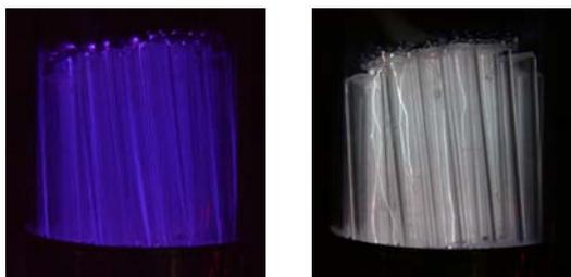
Fig. 4. Images of the discharge in capillaries [diameter 2 mm, length 2 mm] at different AC and DC applied voltages in: (left) ambient air [ $U_{AC} = 15$  kV,  $U_{DC} = -16$  kV], (right) dry nitrogen [ $U_{AC} = 15$  kV,  $U_{DC} = -10$  kV]
