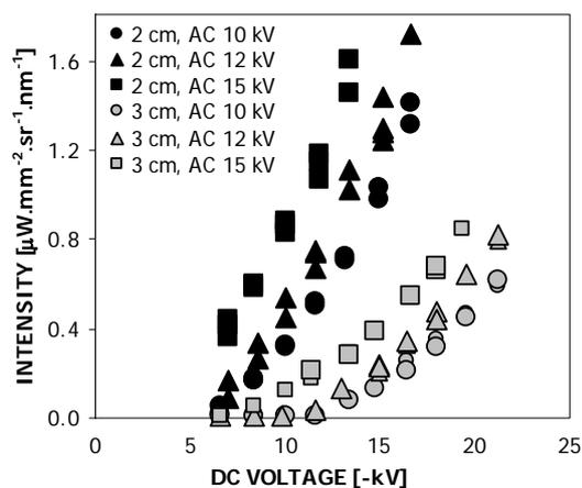
Fig. 6. Discharge emission intensity as functions of negative DC applied voltage for various AC voltage and the length of capillaries [diameter 2 mm, ambient air]
