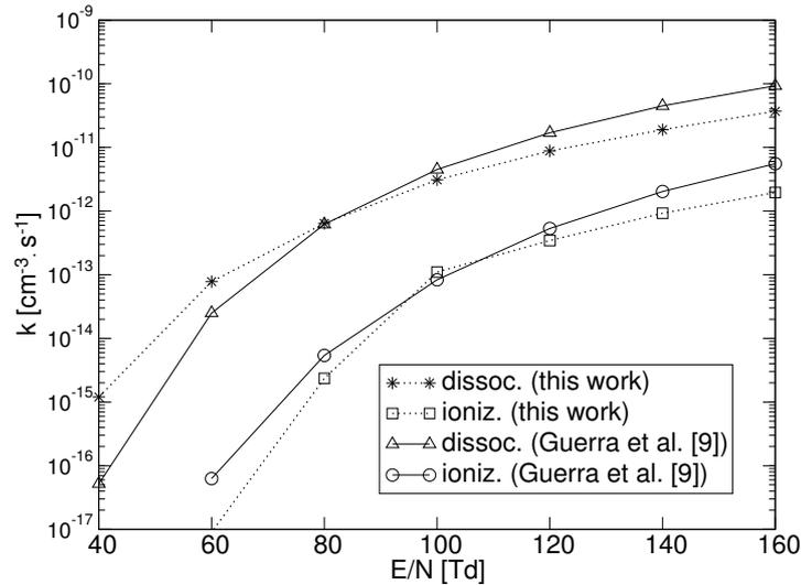
Fig. 4. Rate coefficients of ionization and dissociation of nitrogen.
