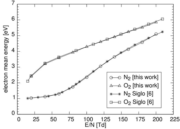
Fig. 2. Electron mean energies in nitrogen and oxygen.
