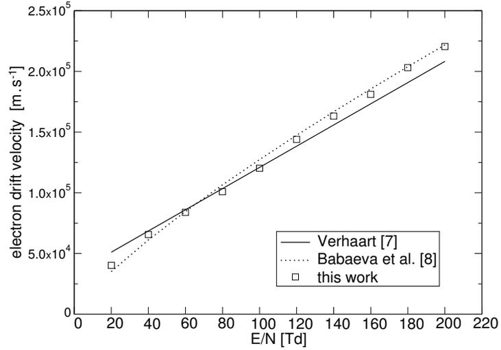
Fig. 3. Electron drift velocity in dry air.
