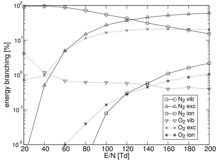
Fig. 5. The branching of electron energy in dry air.
