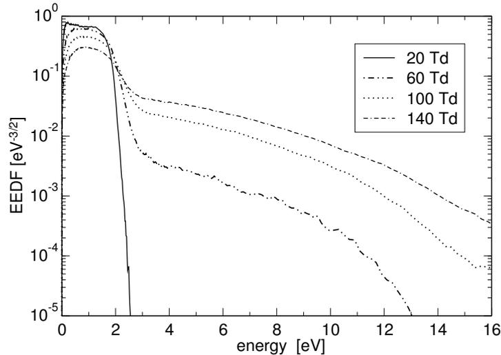
Fig. 1. EEDF in pure nitrogen for different E/N.
