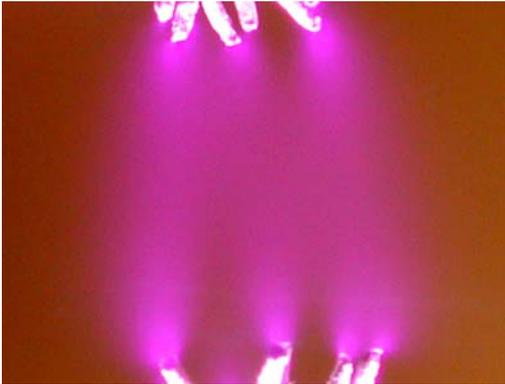
**Figure 11. Multi-pin repetitively pulsed discharge in preheated ( $\sim 2000 \text{ K}$ ), atmospheric pressure air. Discharge volume  $\sim 0.5 \text{ cm}^3$ . Electron number density:  $\sim 10^{12} \text{ cm}^{-3}$ .**
