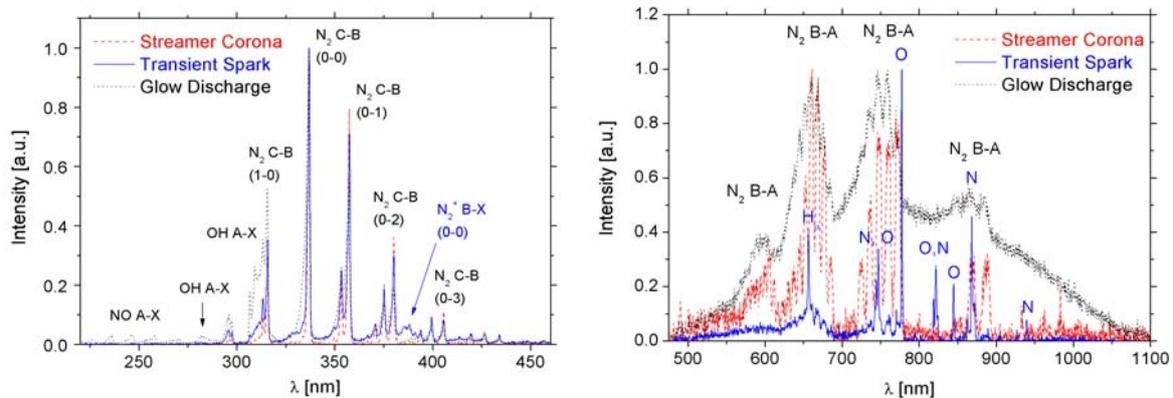
**Figure 4.** Emission spectra of DC discharges in UV and VIS.
