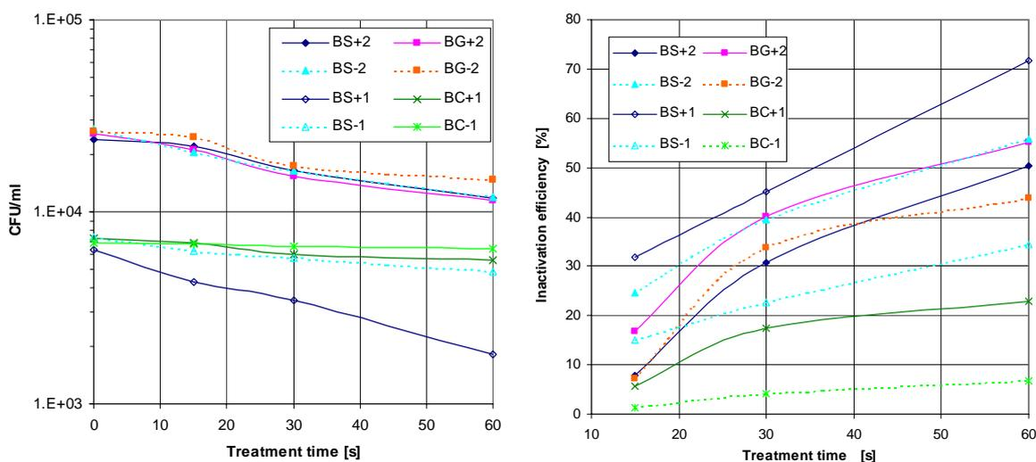
**Figure 6.** *S. typhi* survival curves in semi-logarithmic scale (left) and inactivation efficiency vs. treatment time (right). BS: transient spark, BG: glow discharge, BC: streamer corona, +: positive, -: negative polarity.
