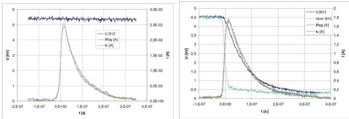
**Figure 3.** Streamer corona (left) and transient spark (right) – voltage and current pulses.  $U_{cor}$  is the voltage corrected for the value of the separating resistor  $r$ ,  $I_{Rog}$  measured by the Rogowski current monitor,  $I_s$  measured by the current probe on a  $50 \Omega$  resistor.
