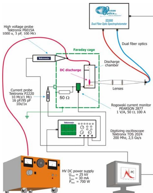
**Figure 1.** Experimental set-up for DC discharge experiments
