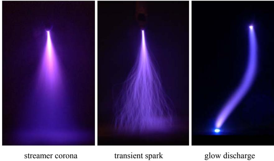
**Figure 2.** Photographs of the discharges at various exposures, gap distance 4 mm.
