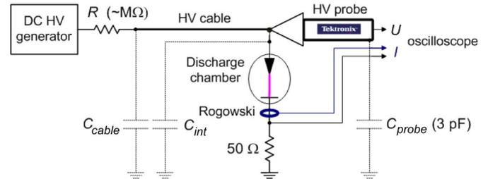
Fig. 1. Schematic of the electrical circuit of dc discharges.
