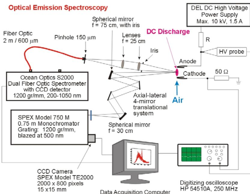
**Figure 1.** Experimental setup for optical emission spectroscopy and electrical measurements of the DC discharges.
