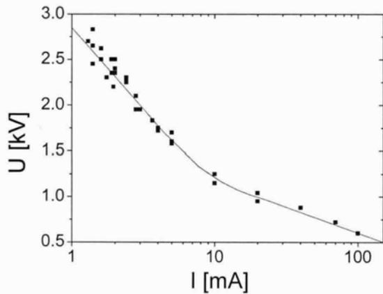
**Figure 2.** Voltage-current characteristic of the DC discharge in ambient air. Interelectrode distance  $d = 7$  mm.
