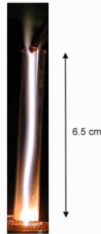
**Figure 6.** DC air discharge with a  $LaCrO_3$  cathode in a glass tube and vortex flow,  $Q = 110$  slpm, tube diameter 8.38 mm,  $I = 500$  mA, discharge diameter 1.8 mm.
