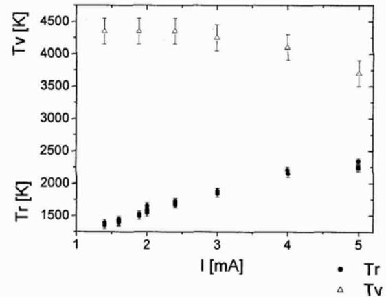
**Figure 5.** Rotational and vibrational temperatures as functions of the discharge current in ambient air at low flow velocity  $v \approx 0.2$  m/s, interelectrode distance  $d = 7$  mm.
