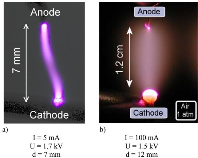
**Figure 4.** DC glow discharges in ambient air flow ( $v = 0.2$  m/s) at atmospheric pressure (different exposure times were used).
