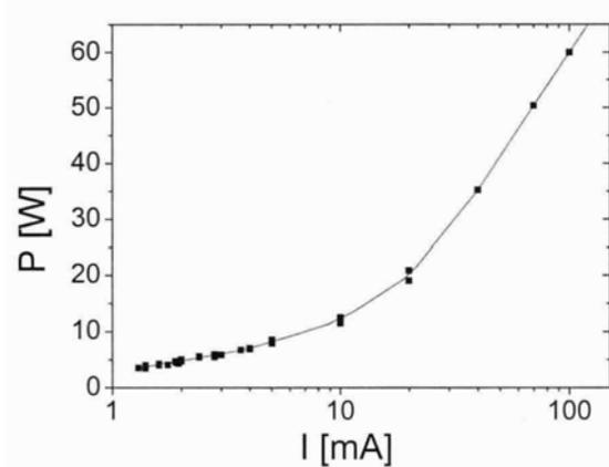
**Figure 3.** Discharge power as a function of current. Interelectrode distance  $d = 7$  mm.
