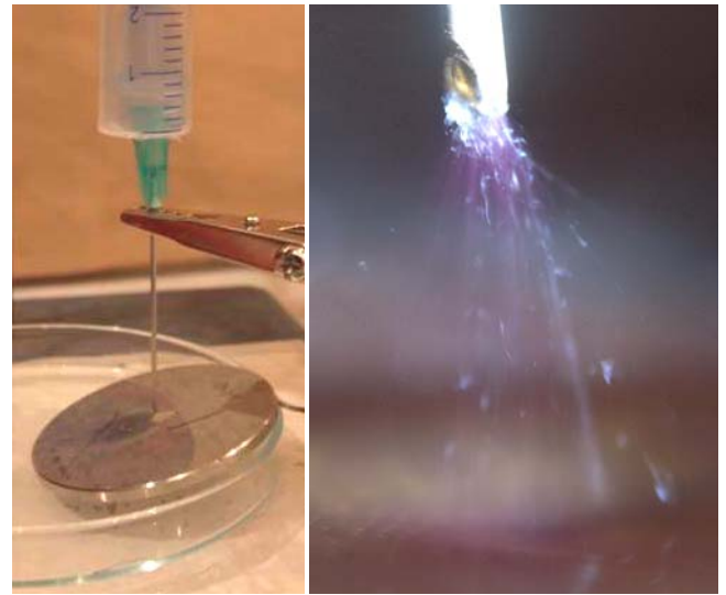
Fig. 3. (Color online) Flowing the contaminated water through the high voltage needle electrode and electro-spraying effect in the corona discharge.
