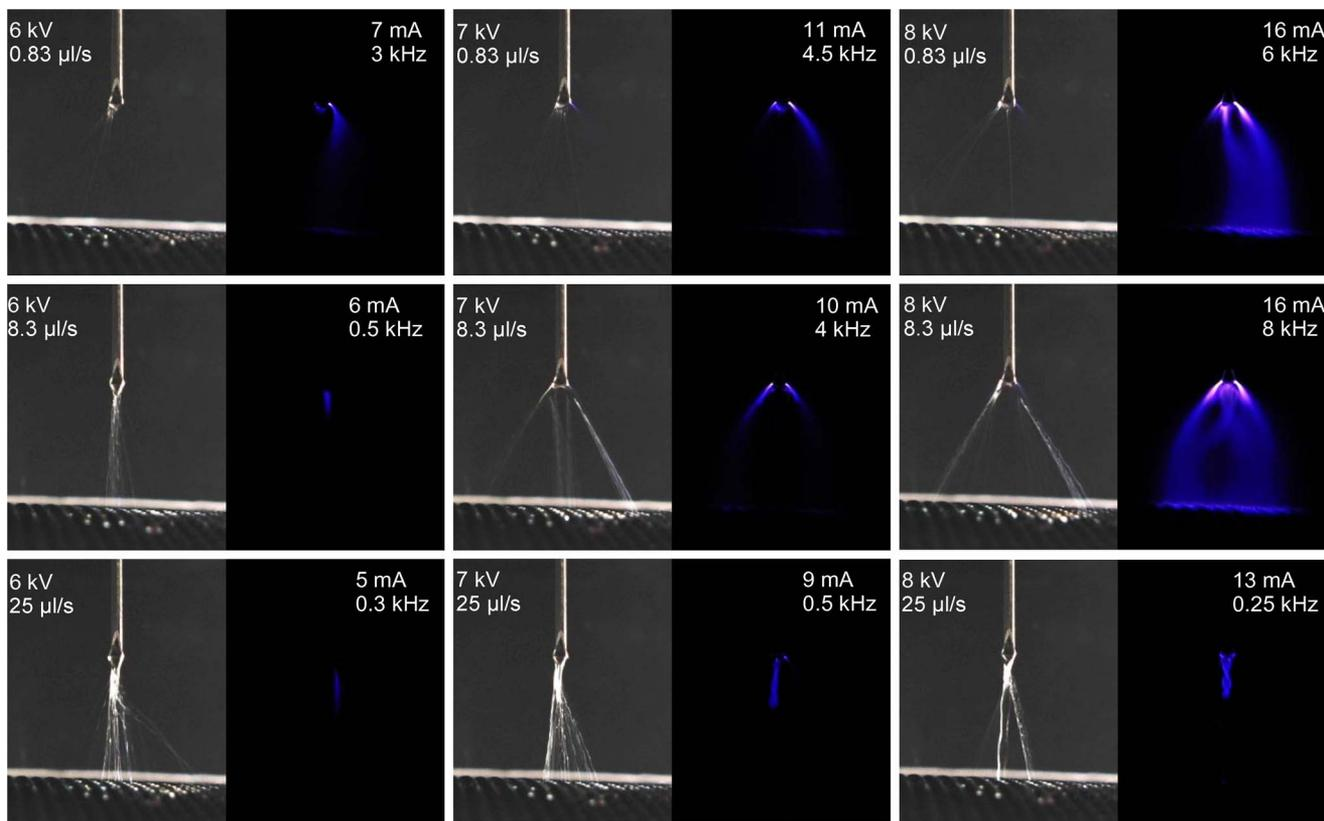
Fig. 1. Electrospaying effect with streamer corona discharge depending on the voltage and the water flow rate with the typical current amplitudes and frequencies ( $d = 1\text{ cm}$ ,  $f/2.7$ ). Exposure time was  $1/15\text{ s}$  for illuminated pictures showing water streams and  $4\text{ s}$  for dark pictures showing discharge regions under the same conditions.
