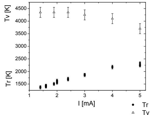
Figure 4. Rotational and vibrational temperatures as functions of the discharge current in ambient air. Flow velocity  $v \approx 0.2$  m/s, interelectrode distance  $d = 7$  mm, positive point-to-plane configuration.
