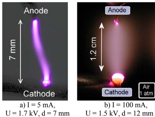
Figure 3. DC discharges in ambient air flow ( $v = 0.2$  m/s) at atmospheric pressure. Platinum pin-to-pin configurations, different exposure times were used.
