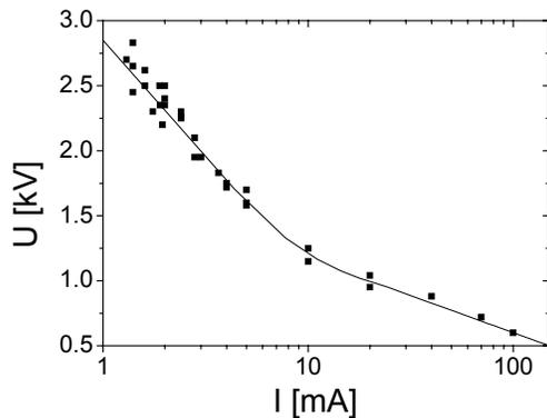
Figure 2. Voltage-current characteristic of the DC discharges in ambient air. Interelectrode distance  $d = 7$  mm, various electrode materials, point-to-plane or pin-to-pin configurations.
