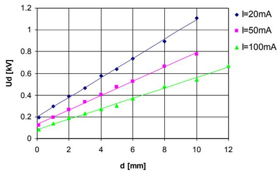
Figure 5. Voltage as a function of interelectrode distance  $d$  for various currents of DC discharges with  $\text{LaCrO}_3$  cathode. The vertical offset on  $U_d$ -axis represents the cathode fall.
