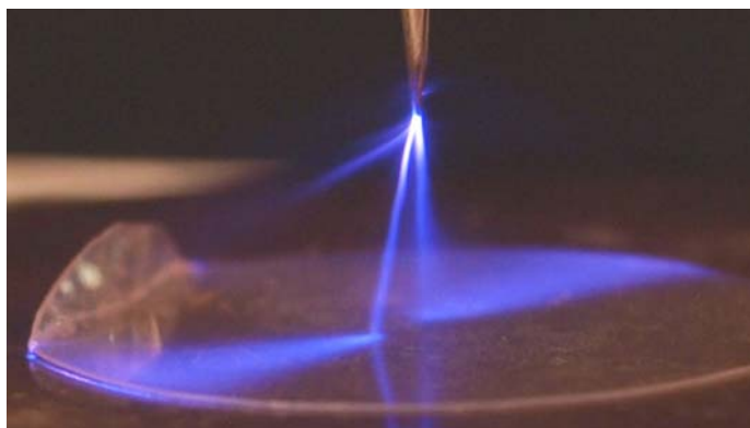
Fig. 1. The positive streamer corona discharge over a polypropylene surface contaminated by spores. U = 6 \text{ kV} , f = 15 \text{ kHz} , I_{\text{max}} = 100 \text{ mA} .
