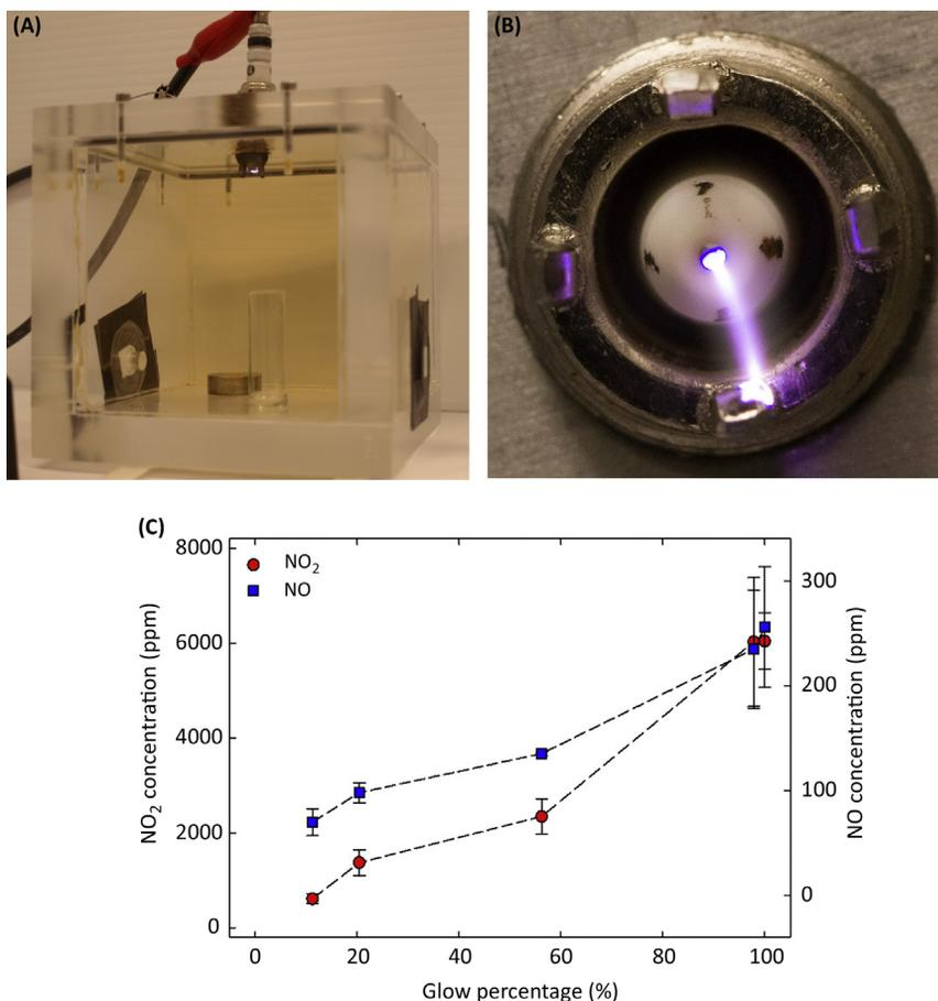
**Figure 2.** 'NOxBox' for Medical Instrument Sterilization by Antimicrobial NO<sub>x</sub>. (A and B) Photographs of the NOxBox with the detail of the hybrid glow-spark air discharge on a spark plug. (C) Temporal evolution of *Escherichia coli* log reductions on stainless steel surfaces and in aqueous saline solution in the NOxBox powered by the quasi-sinusoidal AC waveform from neon-sign transformer. Reproduced, with permission, from [14].
