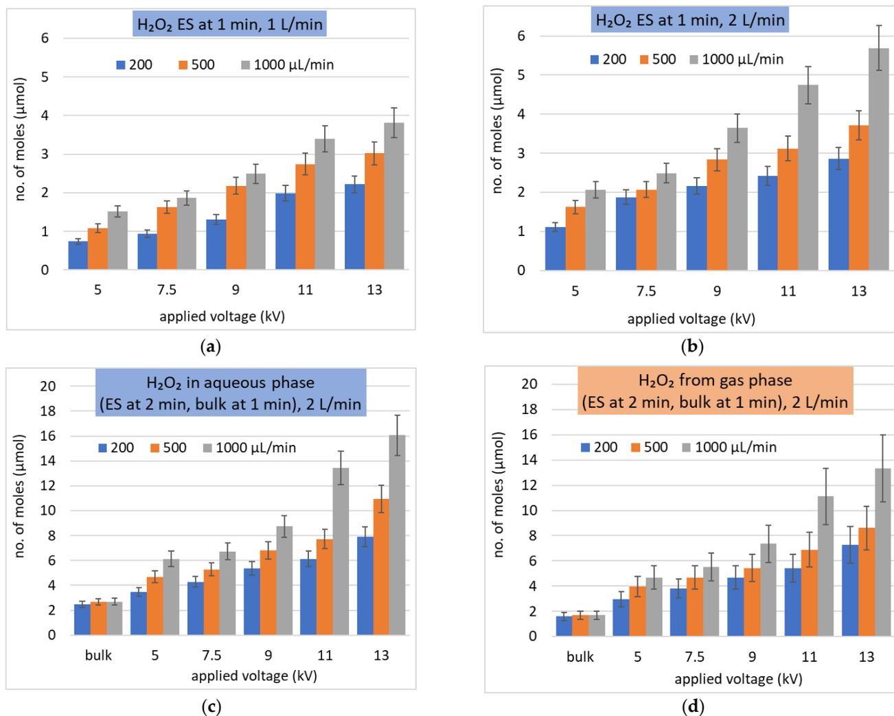
**Figure 8.** Solvation of  $H_2O_2$  as the molar number of dissolved molecules in ES. (a,b) different gas flow rates (L/min) and  $Q_w$  ( $\mu\text{L}/\text{min}$ ) during 1 min treatment time; (b,c) the same gas flow rate 2 L/min and different treatment times (min) in ES and in (c) also bulk water added; (d) depleted  $H_2O_2$  from the gas at the conditions of (c).
