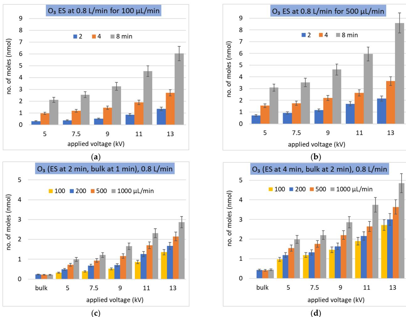
**Figure 7.** Solvation of  $O_3$  as a molar number of dissolved molecules in ES at a constant gas flow rate (L/min). (a,b) two values of constant  $Q_w$  ( $\mu\text{L}/\text{min}$ ) and different treatment times (min); (c,d) different  $Q_w$  ( $\mu\text{L}/\text{min}$ ) during different treatment times (min) in ES and bulk water.
