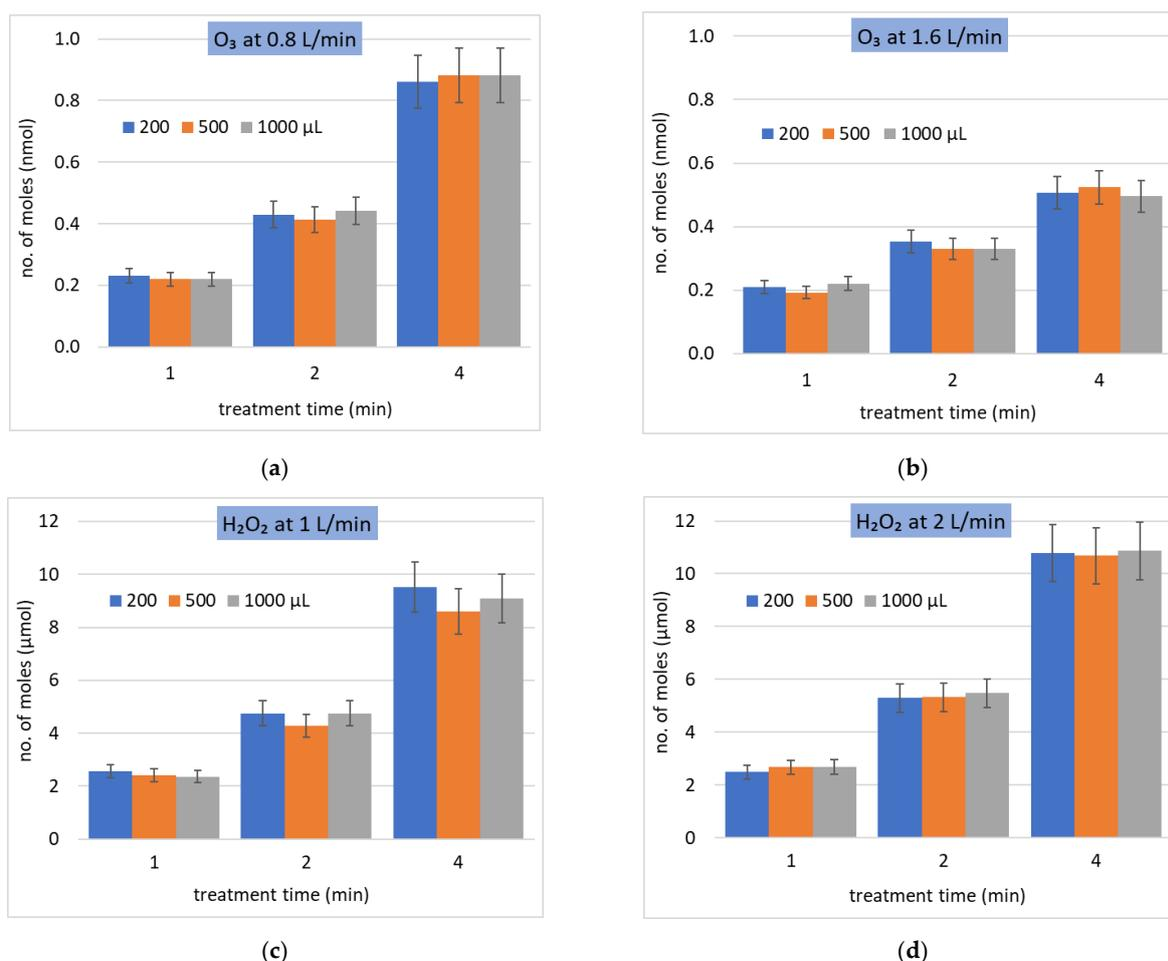
**Figure 3.** Solvation of (a,b)  $O_3$  and (c,d)  $H_2O_2$  at different gas flow rates (L/min) and water volumes ( $\mu$ L) during different treatment times (min) in bulk water. Total molar number of dissolved molecules as a function of treatment time, different water volumes, at constant gas-liquid interface area.
