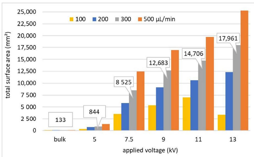
**Figure 6.** The total surface area of water droplets and microdroplets formed by ES during 1 min for different  $Q_w$  ( $\mu\text{L}/\text{min}$ ) as a function of  $V_a$  (kV), compared to the bulk water experiment.
