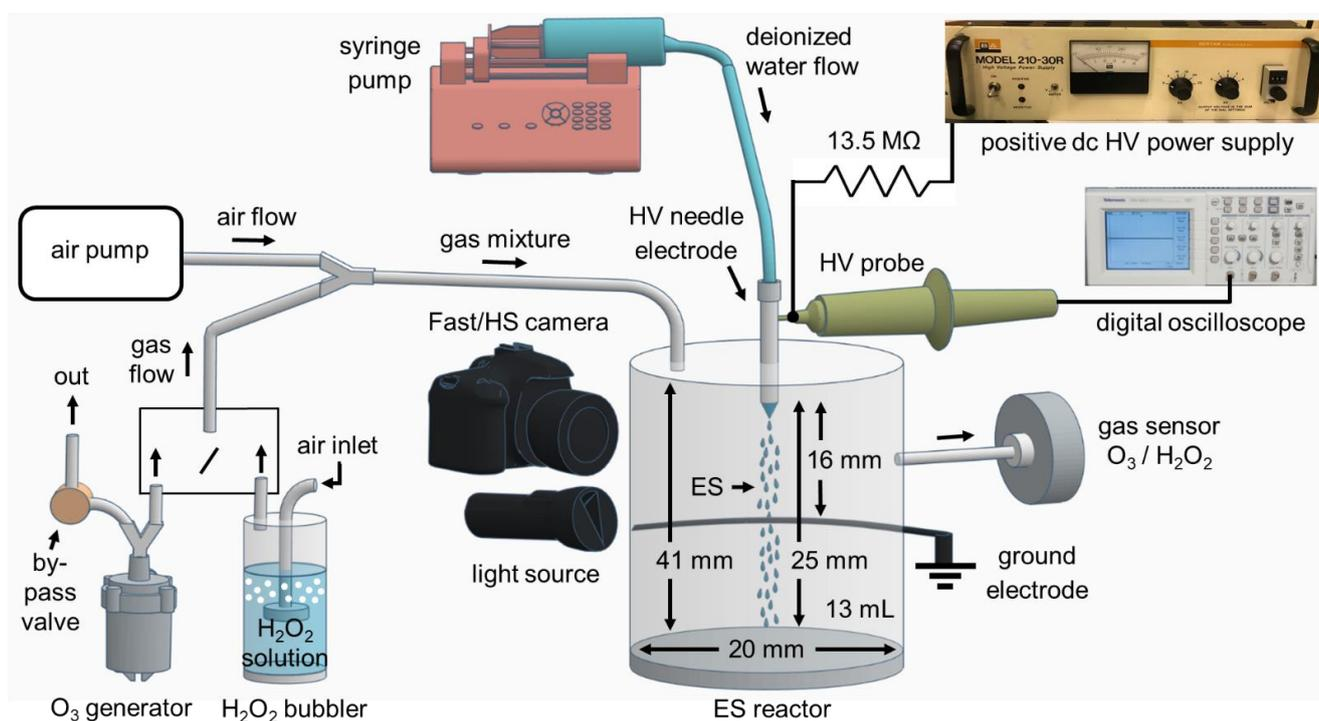
**Figure 2.** Schematic of the experimental setup for the Fast/high speed (HS) camera imaging technique and investigation  $H_2O_2$  and  $O_3$  transport into water electrospay (ES).
