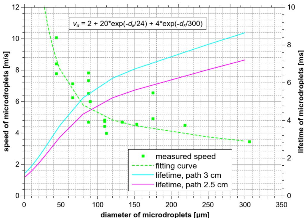
**Figure 11.** Speed of the ES microdroplets measured from the HS camera images and their lifetime as a function of their diameter  $d_k$ .
