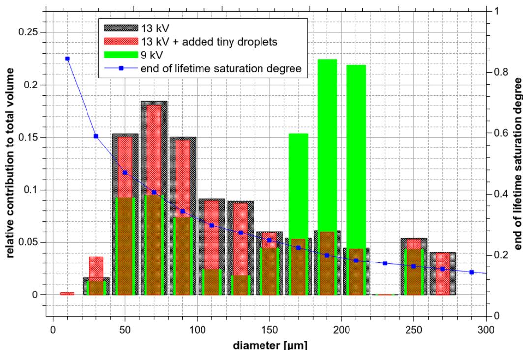
**Figure 13.** Relative contribution of the droplets with different diameters to the total volume  $P^v(d_k)$  and saturation degree at the end of their lifetime  $\zeta^{fin}(d_k)$  as a function of droplet diameter,  $V_a = 9$  and  $13$  kV,  $Q_w = 300$   $\mu\text{L}/\text{min}$ .
