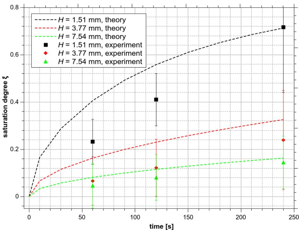
Figure 12. Saturation degree  $\zeta_{O_3}$  of  $O_3$  as a function of treatment time and the bulk water depth  $H$ .
