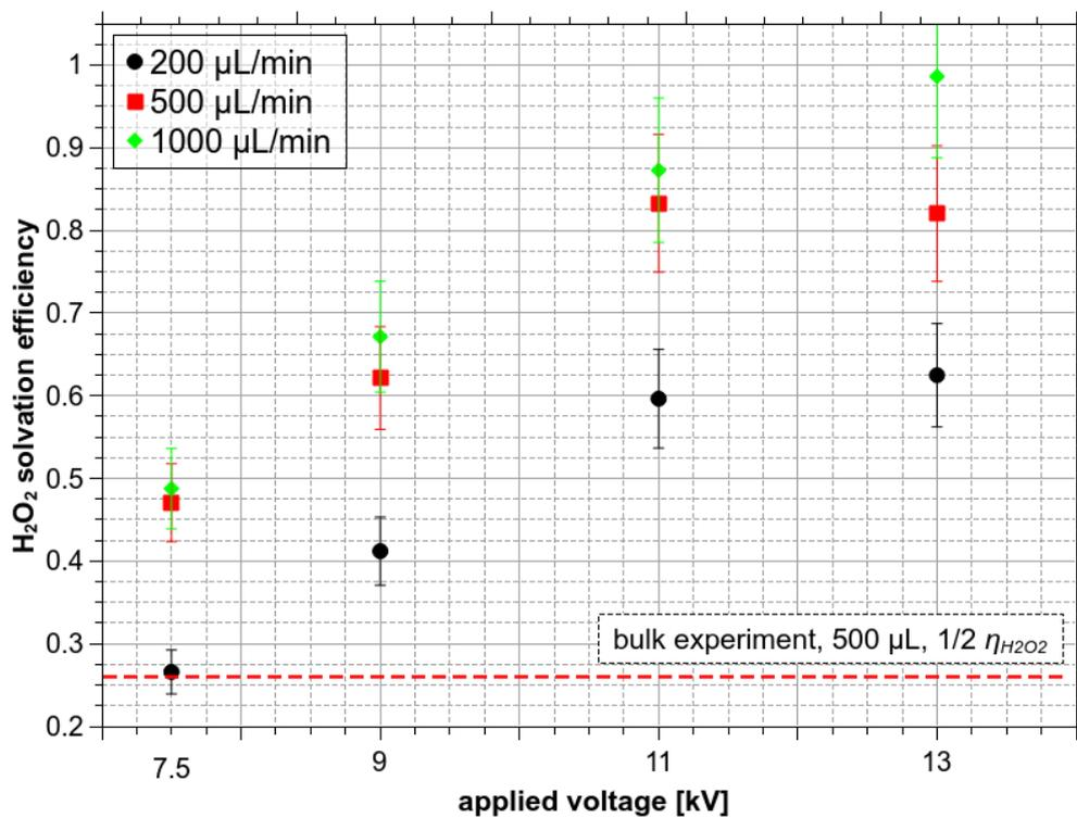
Figure 10. Solvation efficiency of  $H_2O_2$  at a gas flow of 1 L/min as a function of  $V_a$  (kV), treatment time 1 min, at different  $Q_w$  ( $\mu\text{L}/\text{min}$ ).
