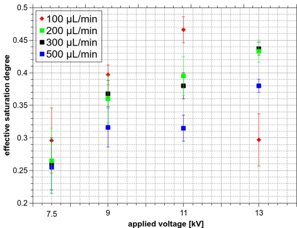
**Figure 14.** Effective  $\text{O}_3$  saturation degree  $\zeta^{\text{eff}}$  of flying microdroplets as a function of  $V_a$  (kV) at different  $Q_w$  ( $\mu\text{L}/\text{min}$ ).
