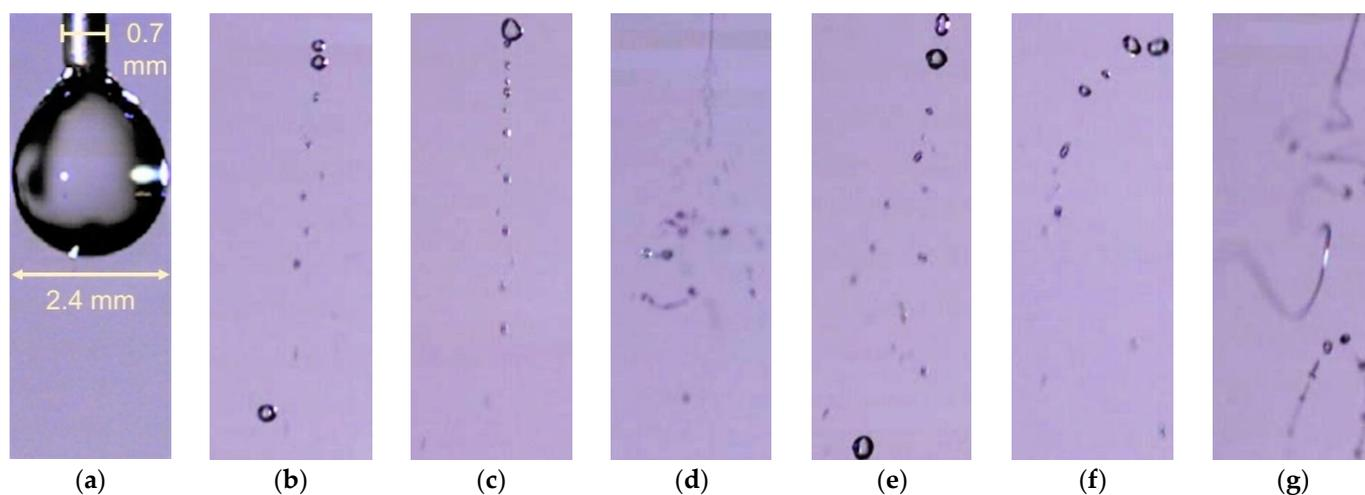
**Figure 4.** Examples of water droplets photographs by HS camera for different  $V_a$  (kV) and  $Q_w$  ( $\mu\text{L}/\text{min}$ ): (a) 0 kV; (b) 9 kV,  $300 \mu\text{L}/\text{min}$ ; (c) 11 kV,  $300 \mu\text{L}/\text{min}$ ; (d) 13 kV,  $300 \mu\text{L}/\text{min}$ ; (e) 9 kV,  $500 \mu\text{L}/\text{min}$ ; (f) 11 kV,  $500 \mu\text{L}/\text{min}$ ; (g) 13 kV,  $500 \mu\text{L}/\text{min}$ .
