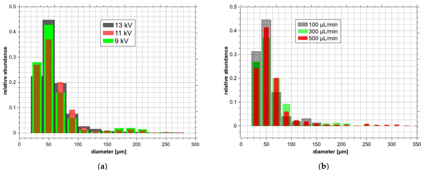
**Figure 5.** The relative abundance of water microdroplets produced by ES as a function of microdroplets diameter at different  $V_a$  (kV) and  $Q_w$  ( $\mu\text{L}/\text{min}$ ): (a) 9, 11, 13 kV, and 300  $\mu\text{L}/\text{min}$ ; (b) 11 kV and 100, 300, 500  $\mu\text{L}/\text{min}$ . Microdroplets with a diameter under 20  $\mu\text{m}$  are below the detection limit of the used camera imaging technique.
