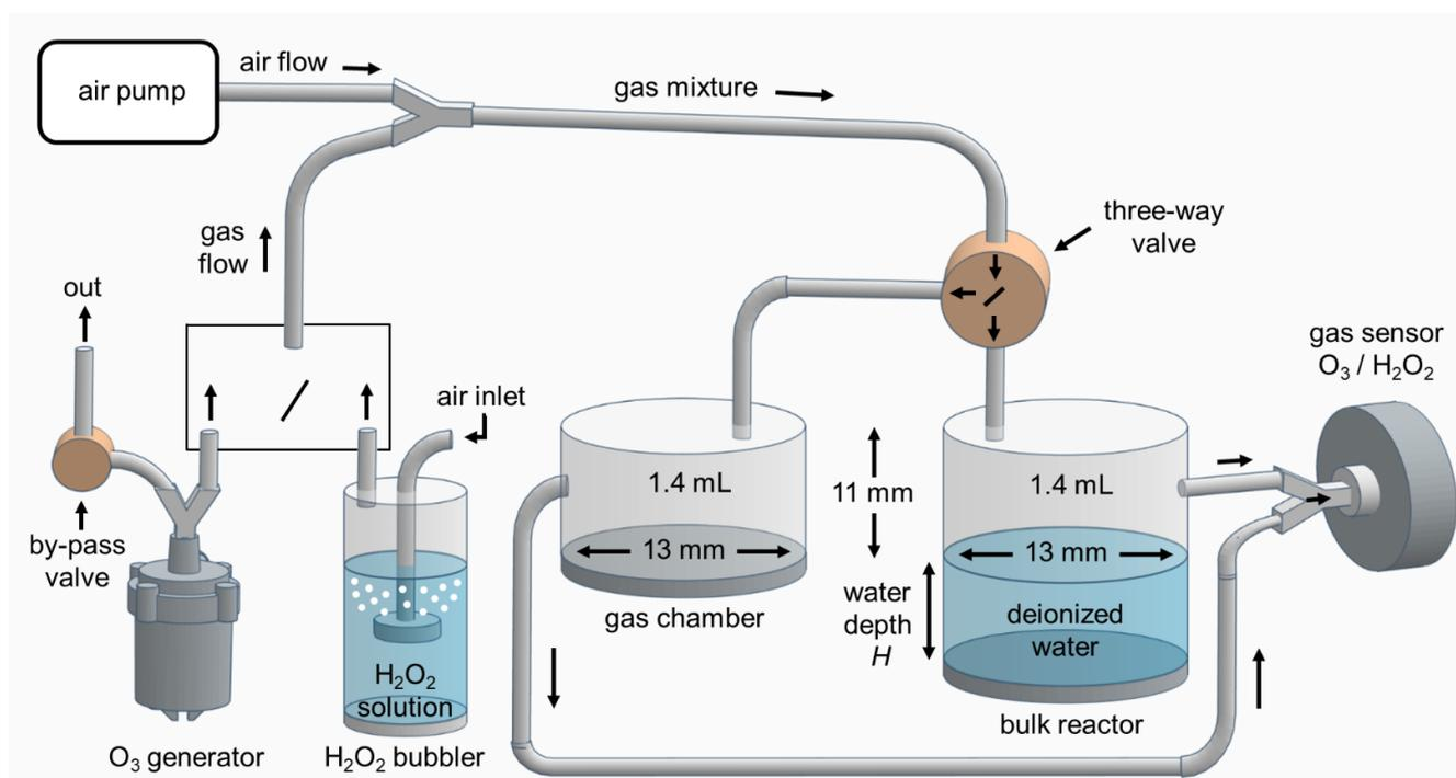
**Figure 1.** Schematic of the experimental setup for investigation H<sub>2</sub>O<sub>2</sub> and O<sub>3</sub> transport into bulk water.
