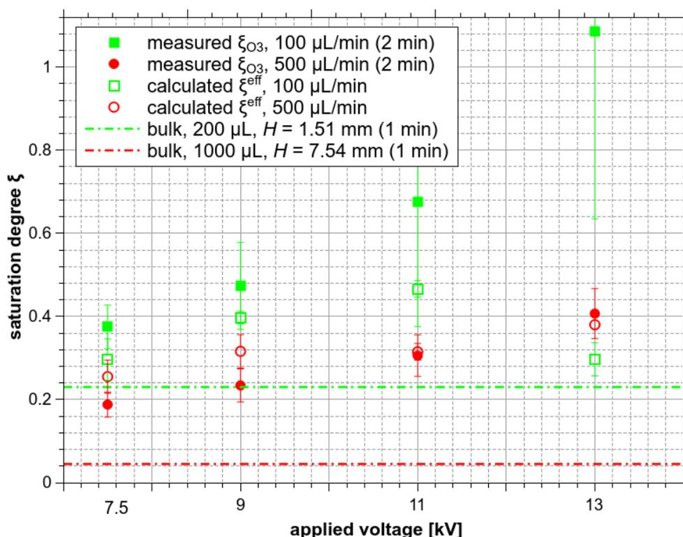
**Figure 15.** Comparison of  $O_3$   $\zeta^{eff}$  calculated from the size distribution histograms (Figure 5) of flying microdroplets with the measured  $\zeta_{O_3}$  of bottom microdroplets of two sets of ES experiments ( $Q_w = 100$  and  $500 \mu\text{L}/\text{min}$ ), and  $O_3$  saturation in the corresponding bulk experiments.
