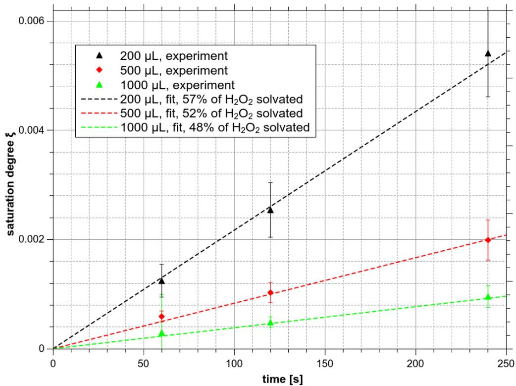
Figure 9. Saturation degree  $\xi_{H_2O_2}$  of  $H_2O_2$  as a function of treatment time and bulk water volume.
