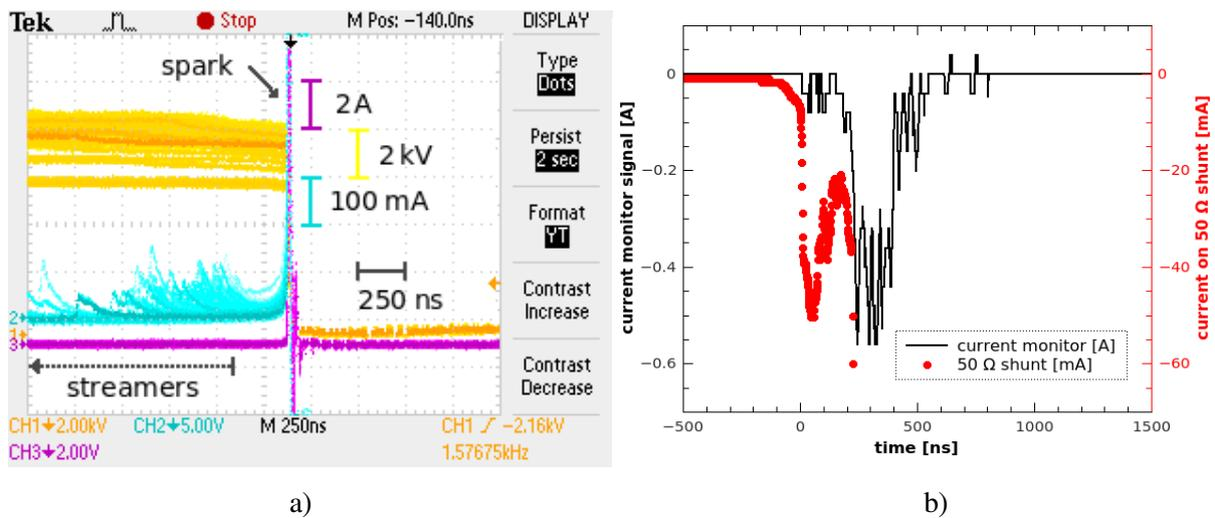
Fig. 3. Accumulated negative polarity TS waveforms (persist 2 s) triggered on spark current pulse, all signals inverted (a), and averaged TS current waveforms (128 pulses) triggered on the beginning of the streamer (b).
