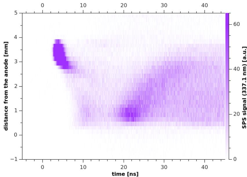
Fig. 5. Cross-correlation spectroscopy record of the TS evolution, negative polarity, cathode at the top, repetition rate  $\sim 2$  kHz, gap 4 mm, SPS emission signal rescaled, with initial phase saturated.
