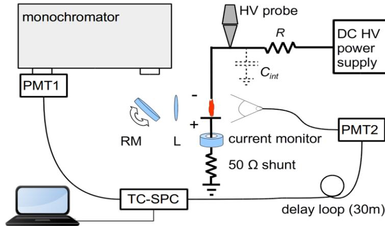
Fig. 1. Schematic of the experimental setup, PMT – photo multiplier, TC-SPC – time correlated single photon counting board, RM – rotating mirror, L – lens, R – external resistor.
