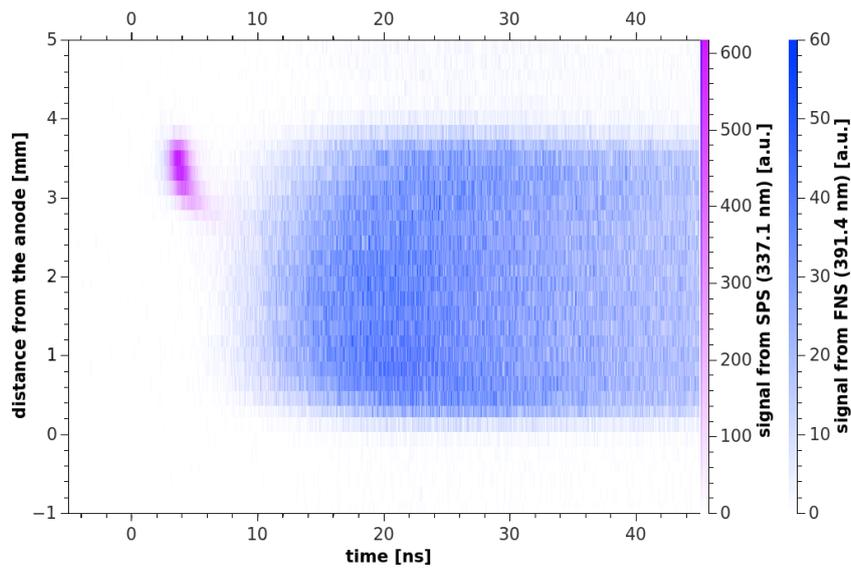
Fig. 4. Cross-correlation spectroscopy record of the TS evolution, negative polarity, cathode at the top, repetition rate  $\sim 2$  kHz, gap 4 mm, overlapped signal from the SPS and FNS emission.
