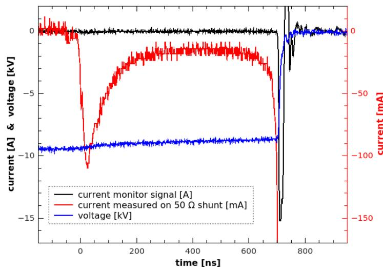
Fig. 2. Typical negative polarity TS waveforms, single pulse, repetition rate ~ 2 kHz,  $C_{int}$  ~ 30 pF.
