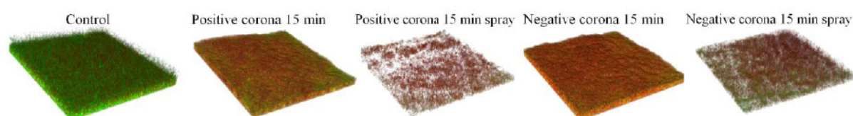
Fig. 2: Three-dimensional reconstruction of the biofilm z-stacks from CLSM. Red indicates dead cells and green live cells. From the left: control dried 20 min at 35°C, DC corona discharge treated samples for 15 min with or without water electrospray (magnification 60×, section size 211.2×211.2 μm).
