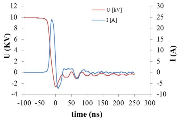
Fig. 2. The typical voltage and current pulse waveforms of the transient spark with water electro spray
