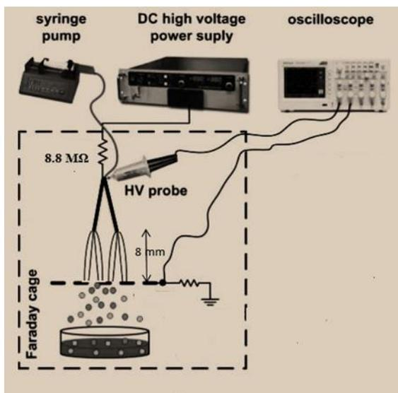
Fig. 1. The experimental setup with electro-spray of water through two needles and two parallel transient spark discharges
