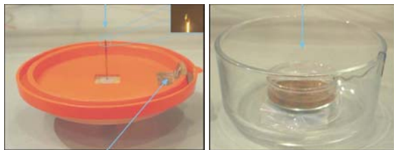
Fig. 4. Single needle – Petri dish discharge chamber for static water treatment
