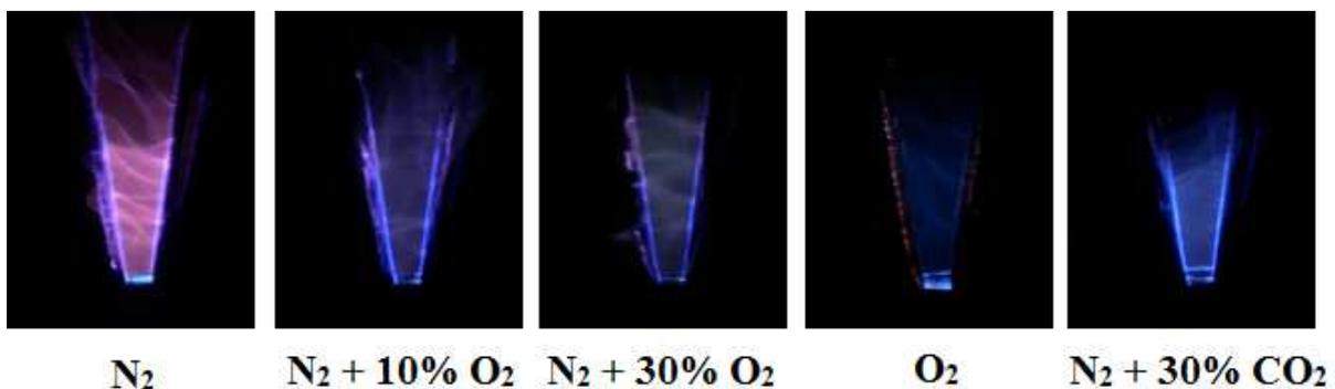
Fig. 3. Effect of gas mixture (exposure time 1/4 s).
