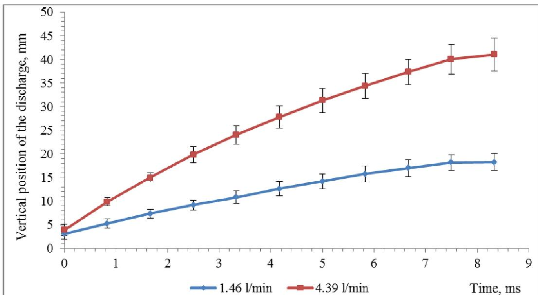
Fig.7. Uncertainty of measurement as the standard deviation for two flow rates (N<sub>2</sub>).
