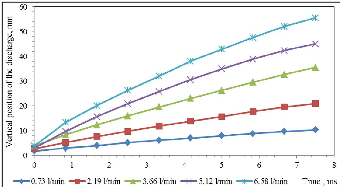
Fig. 6 Vertical position of the discharge propagation for different flow rates (N<sub>2</sub>).
