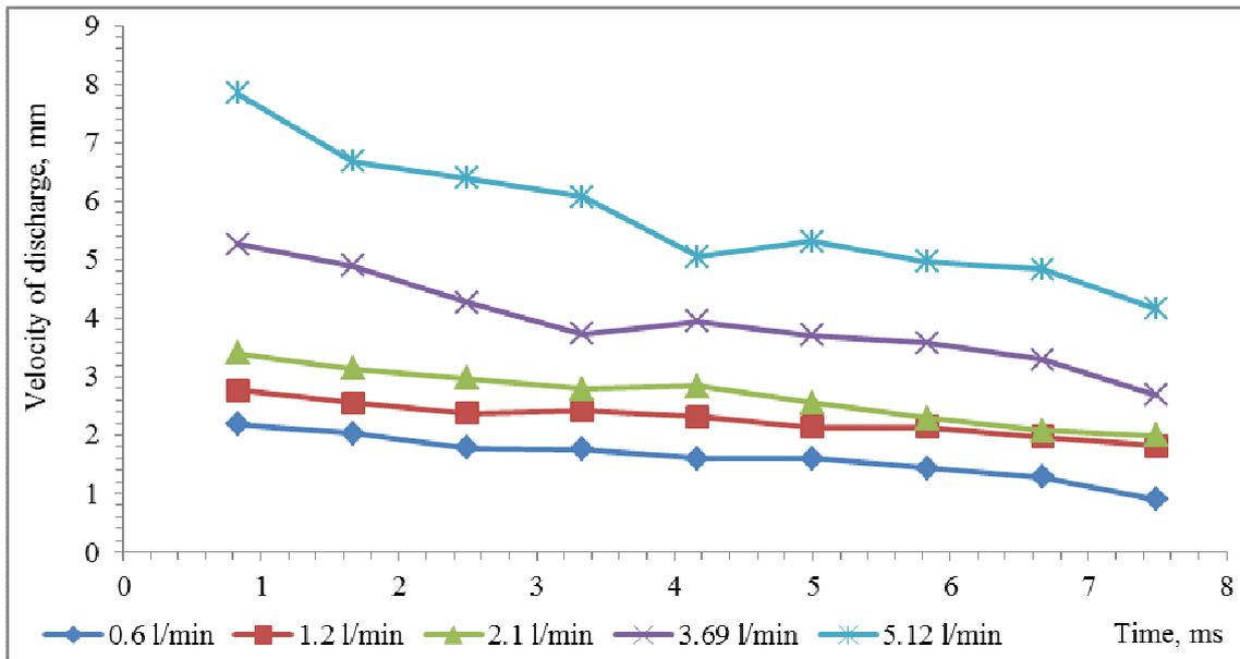
Fig. 8. Velocity of discharge for different flow rates (O<sub>2</sub>).
