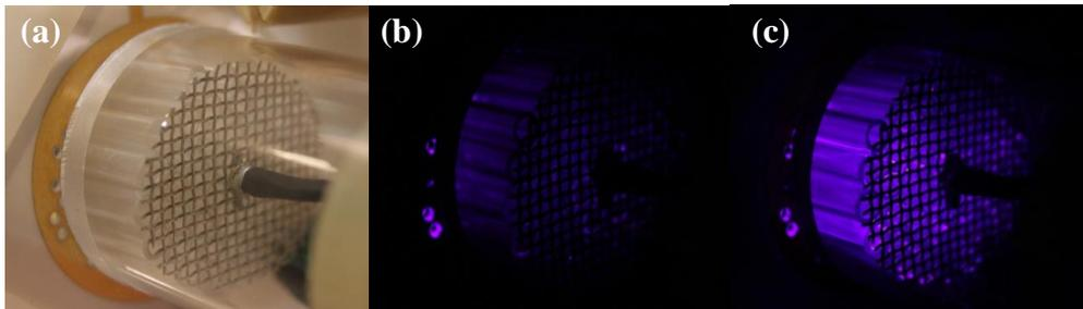
Fig. 3. The ceramic substrate with glass capillaries: (a) without discharge; (b) with applied AC HV (4 kV @ 1 kHz); (c) with applied both AC and DC HV (4 kV @ 1 kHz; +16 kV, respectively) (ambient air, 2.4 L/min) (Exposure time 4 s, f/5.6, ISO 400).
