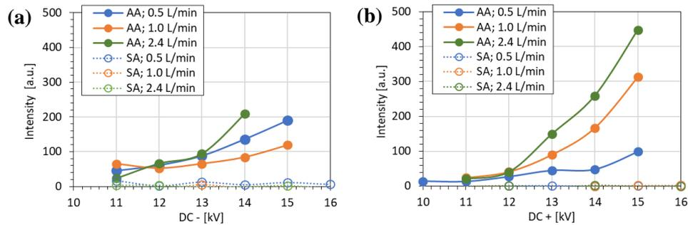
Fig. 4. Emission intensity of the capillary discharge as a function of amplitude of the applied (a) negative or (b) positive DC HV in ambient air (AA) and synthetic air (SA) with various flow rates (0.5; 1.0 and 2.4 L/min).
