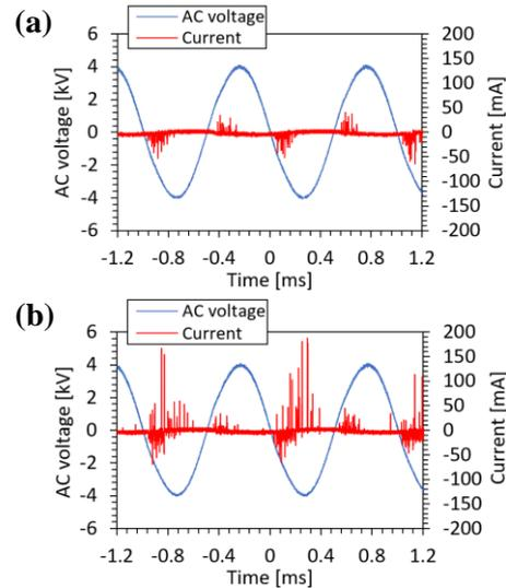
Fig. 2. Voltage and current waveforms of (a) surface barrier discharge (AC HV 4 kV @ 1 kHz) and (b) capillary discharge (AC HV 4 kV @ 1 kHz; DC HV +16 kV; R 9.4 MΩ).
