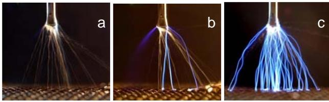
**Figure 1.** Photographs of the electro-spray of water in 8 mm gap, water flow rate 0.5 mL/min: (a) electro-spray with SC, 6.5 kV, (b) transition SC-TS, 7.8 kV, (c) spray with TS, 9 kV.
