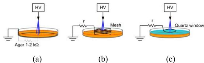
**Figure 2.** Electrode arrangements for (a) direct and (b, c) indirect plasma treatment of contaminated agar plates. (b) Mesh electrode  $\sim 2$  mm above agar surface trapped the charged particles and shielded the electric field. (c) Quartz (or  $\text{MgF}_2$ ) window transmitted only light from the discharge (UV).
