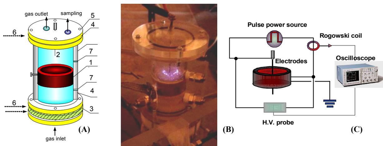
**Figure 1.** (A) Cylindrical foaming column. 1,2- electrodes, 3- ceramic diffuser, 4- housing, 5-bolts, 6-orings, 7- foam level control. (B) The photo of reactor. (C) The electrical pulse power supply.
