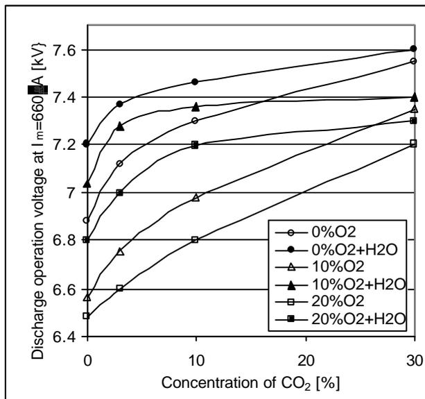
Fig.2: Effect of H<sub>2</sub>O and other gas components of the N<sub>2</sub>-NO-O<sub>2</sub>-CO<sub>2</sub>-H<sub>2</sub>O mixtures on the operating voltage of the discharge at I<sub>m</sub>=660 μA
