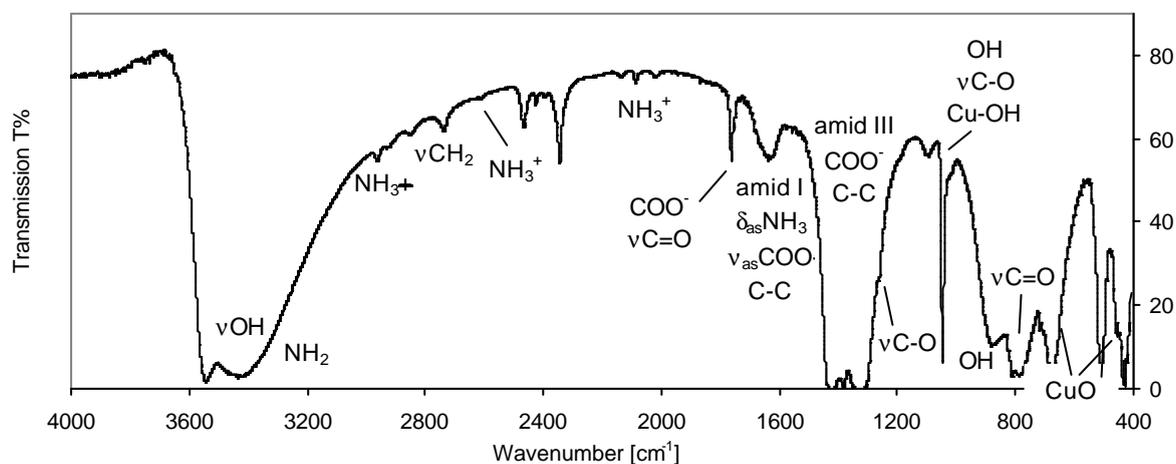
**Fig. 6** IR absorption spectra of solid product formed on the electrode during the measurements in  $\text{N}_2\text{-NO-O}_2\text{-CO}_2$  system treated by positive corona discharge
