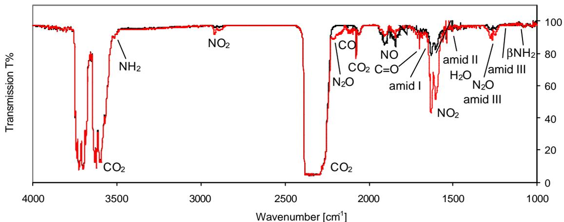
**Fig. 5:** Typical IR absorption spectra of gas mixture treated by positive corona discharge at  $I_m=1000\mu\text{A}$  (N<sub>2</sub> + 500 ppm NO + 10% O<sub>2</sub> + 10% CO<sub>2</sub>)
