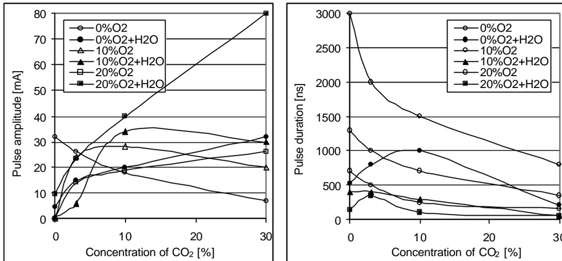
**Fig.4:** Effect of H<sub>2</sub>O and other gas components on the discharge current pulse waveform characteristic, its amplitude (left) and duration (right) at  $I_m=660\mu\text{A}$
