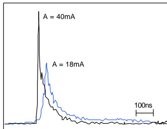
Fig.3: Effect of H<sub>2</sub>O on the discharge current waveform characteristic in the mixture of N<sub>2</sub>-NO-20%O<sub>2</sub>-10%CO<sub>2</sub> at I<sub>m</sub>=660 μA
